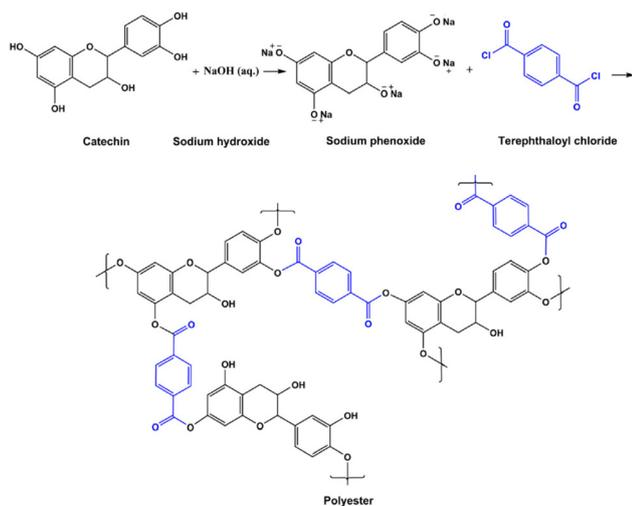
Fig. 3 The IP reaction between catechin and TPC, yielding polyester.<sup>52</sup>
