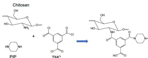
Fig. 6 The IP reaction between chitosan and PIP with TMC to produce polyamide.<sup>74</sup>
