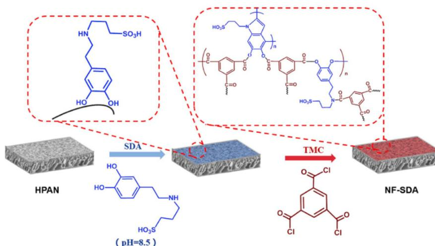
Fig. 7 Preparation of NF membranes by IP, using sulfonated dopamine (SDA) and TMC as monomers.<sup>80</sup>
