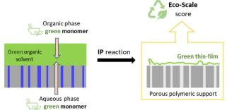
Fig. 2 A schematic representation of the review's concept: summarizing the 'green' options for monomers and organic solvents to perform IP, the corresponding properties of the resultant TFC membrane fabricated, and presenting the 'eco-scale score' calculation for the fabricated membranes
