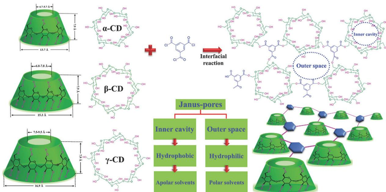
Fig. 5 Chemical structures and architectures of the crosslinked cyclodextrins and TMC, to produce molecular sieving nanofilms by IP.<sup>70</sup>
