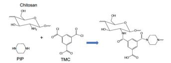
Fig. 6  $\,$  The IP reaction between chitosan and PIP with TMC to produce polyamide.  $^{74}$
