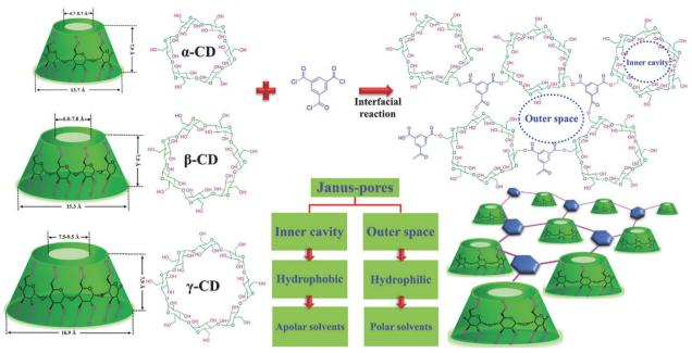
Fig. 5 Chemical structures and architectures of the crosslinked cyclodextrins and TMC, to produce molecular sieving nanofilms by IP.<sup>70</sup>
