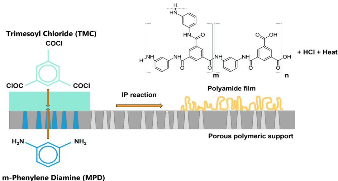
Fig. 1 IP reaction between MPD in the aqueous phase and TMC in the organic phase producing cross-linked polyamide, HCl and heat are by-products.<sup>15</sup>
