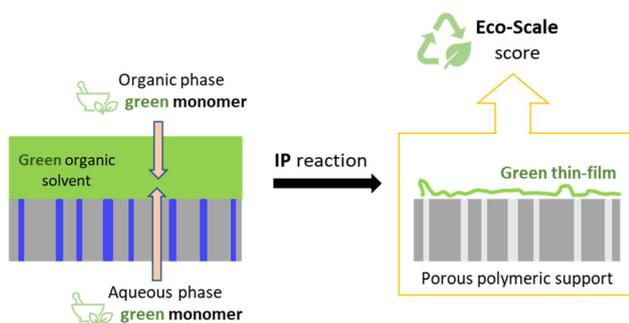
**Fig. 2** A schematic representation of the review's concept: summarizing the 'green' options for monomers and organic solvents to perform IP, the corresponding properties of the resultant TFC membrane fabricated, and presenting the 'eco-scale score' calculation for the fabricated membranes.
