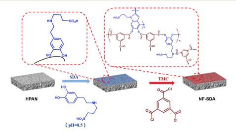
Fig. 7 Preparation of NF membranes by IP, using sulfonated dopamine (SDA) and TMC as monomers. 80
