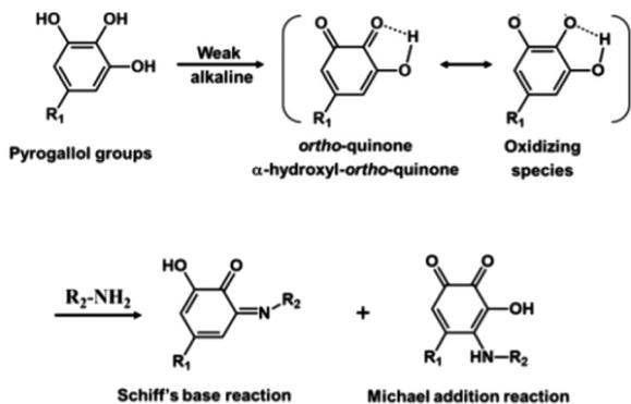
Fig. 8 Reaction mechanism between pyrogallol groups of TA and amine groups of priamine.<sup>61</sup>
