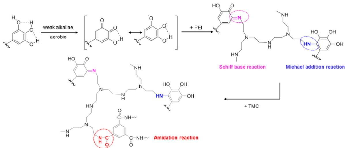
Fig. 4 Reaction mechanism between pyrogallol groups of EGCG, amine groups of PEI, and acyl-chloride.<sup>67</sup>
