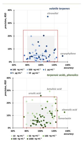
Fig. 2 Accuracy and precision determined at 5 concentration levels for individual analytes. The grey square corresponds to the area covering precision in the range of 0–20% expressed as RSD and accuracy in the range of 80–120%. A red square expresses 25% RSD and accuracy in the range of 75–125%.
