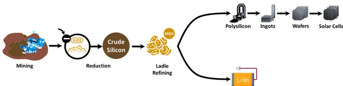
Fig. 4 The supply chain of solar cells and Li-ion batteries with Si anodes.
