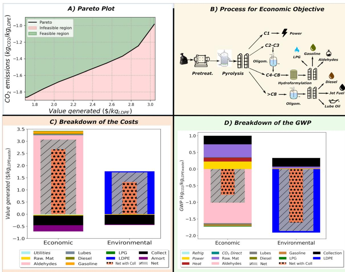
**Fig. 4** Results for the economic and environmental minimization of the GWP. (A) Results at the Pareto frontier. (B) Process flowsheets designed with economic and environmental optimization. (C) Breakdown of the costs. (D) Breakdown of the GWP, where the positive emissions are the emissions generated and the negative are the credits obtained by substituting petrol-based products.
