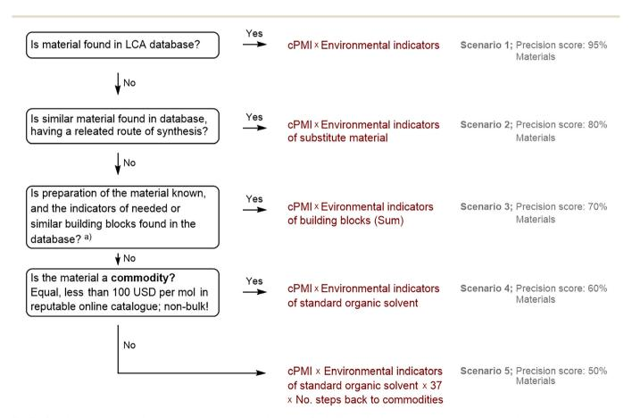
Fig. 3 Calculation of a process' environmental impact using the material's cPMI contribution times their environmental indicators.
