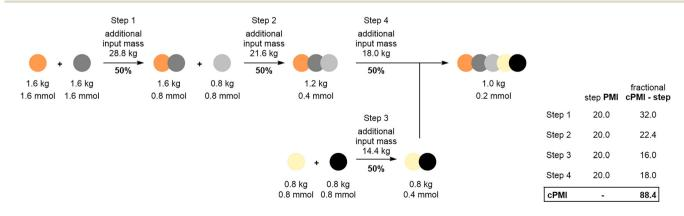
Fig. 1 Example (step) PMI, fractional cPMI - step, and cPMI.
