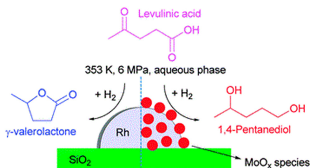
Fig. 1 LA hydrogenation to 1,4-PDO over Rh/MoO x /SiO 2 . Reproduced from ref. 38 with permission from the Royal Society of Chemistry, copyright (2014).
