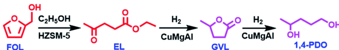
Scheme 5 Reaction pathway for the conversion of FAL into 1,4-PDO over HZSM-5 and CuMgAl catalysts. EL: ethyl levulinate. Reproduced from ref. 85 with permission from the Royal Society of Chemistry, copyright (2022).
