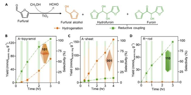
Fig. 20 Photocatalytic conversion of FAL over TiO<sub>2</sub> nanocrystals. (A) Structures of products from hydrogenation of C=O group and reductive coupling of FAL. Variations of product yield and selectivity with time over (B) A-bipyramid, (C) A-sheet, and (D) R-rod. Reproduced from ref. 28, with permission of Elsevier, Copyright 2020.
