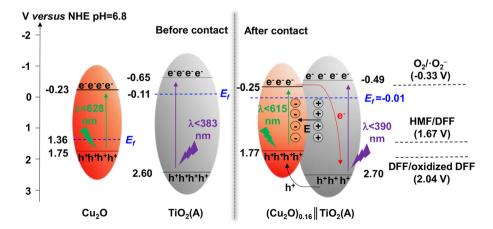
Fig. 3 Schematic illustration of energy band and charge transfer process of the Z-scheme (Cu<sub>2</sub>O)<sub>0.16</sub>||TiO<sub>2</sub>(A) photocatalyst. Reproduced from ref. 45, with permission of Elsevier, Copyright 2023.
