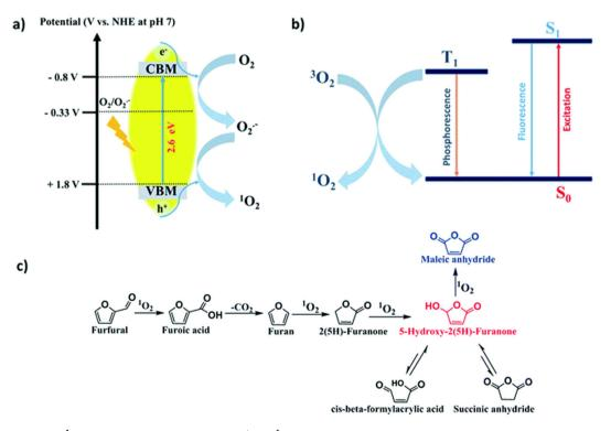
Fig. 22 (a) Generation of <sup>1</sup>O<sub>2</sub> on the surface of SGCN via h<sup>+</sup>, (b) <sup>1</sup>O<sub>2</sub> generation via triplet state energy transfer, and (c) plausible mechanistic pathway of FAL photooxidation. Reproduced from ref. 36, with permission of Royal Society of Chemistry, Copyright 2022.
