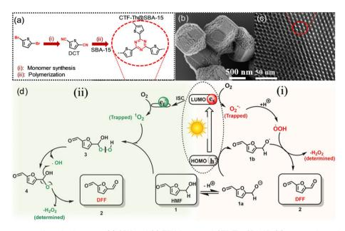
Fig. 8 (a) Chemical structure and synthesis routes, (b) SEM and (c) TEM images of CTF-Th@SBA-15, (d) proposed reaction mechanism for the photocatalytic partial oxidation of HMF to DFF using CTF-Th@SBA-15 via two possible routes using either  ${}^{1}O_{2}$  or  ${}^{1}O_{2}$ . ISC: Inter System Crossing. Reproduced from ref. 26, with permission of John Wiley & Sons, Inc, Copyright 2020.
