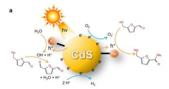
Fig. 14 Schematic mechanism for selective photocatalytic oxidation of HMF to DFF or HMFCA by the Ru CdS catalyst. Reproduced from ref. 60, with permission of John Wiley & Sons, Inc, Copyright 2022.
