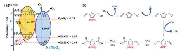
Fig. 15 (a) Schematic diagram of  $e^--h^+$  pair separation over the  $g-C_3N_4/NaNbO_3$  heterojunction. (b) Proposed mechanism for the  $g-C_3N_4/NaNbO_3$ NaNbO<sub>3</sub>-catalyzed oxidation of HMF under visible light. Reproduced from ref. 105, with permission of Elsevier, Copyright 2020.
