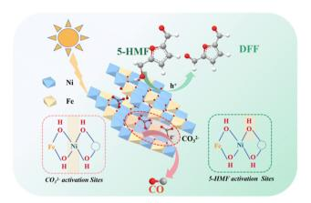
Fig. 11 Proposed mechanism of the integration of CO<sub>2</sub> photoreduction with oxidation of HMF. Reproduced from ref. 33, with permission of Royal Society of Chemistry, Copyright 2023.
