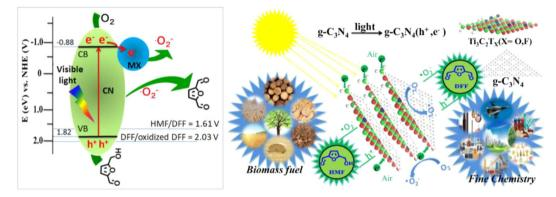
Fig. 4 Illustration of the mechanism for selective photooxidation of HMF into DFF over the  $Ti_3C_2/g$ - $C_3N_4$  catalyst under visible light irradiation. Reproduced from ref. 23, with permission of Elsevier, Copyright 2020.
