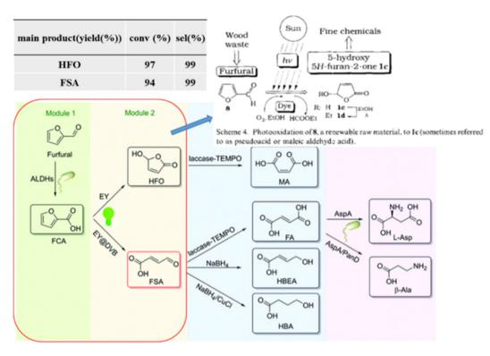
Fig. 21 Schematic illustration of photocatalytic FAL to HFO over organic dye. Reproduced from ref. 35, with permission of John Wiley & Sons, Inc., Copyright 1994. Organic dye combined with biological and chemical photocatalysts for FAL to HFO or FSA. Reproduced from ref. 38, with permission of Royal Society of Chemistry, Copyright 2021.
