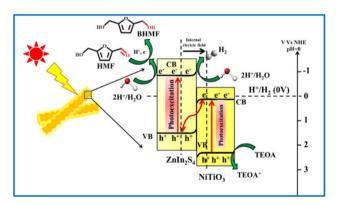
Fig. 18 Pictorial representation of Z-scheme mechanism for photocatalytic H<sub>2</sub> generation and subsequent HMF reduction by NiTiO<sub>3</sub>/ ZnIn<sub>2</sub>S<sub>4</sub> hierarchical nanostructures. Reproduced from ref. 113, with permission of Elsevier, Copyright 2022.
