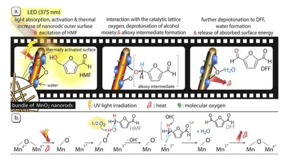
Fig. 7 Illustrated representation of the light effect and the involved oxidation mechanism of HMF over the MnO<sub>2</sub>-NRs photocatalyst. Reproduced from ref. 76, with permission of Elsevier, Copyright 2019.
