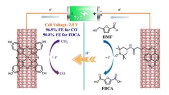
Fig. 12 Schematic diagram of sunlight-driven paired electrolysis of the CO₂RR and HMFOR by the TBP-CoPc/Py-TEMPOs photocatalyst. Reproduced from ref. 98, with permission of Royal Society of Chemistry, Copyright 2022.
