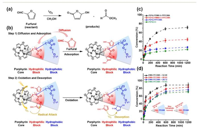
Fig. 23 (a) Scheme for oxidation of FAL, (b) detailed reaction mechanism of FAL oxidation utilizing amphiphilic block copolymer, reaction kinetics for FAL oxidation, (c) using porphyrin-based copolymers, and (d) using P(Pd)-PDMA-PPEGMA with varying block fraction. Reproduced from ref. 133, with permission of Elsevier, Copyright 2022.
