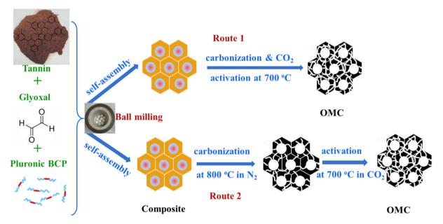
Fig. 14 Diagrammatic representation of the two processes used in the mechanochemical synthesis of OMCs: carbonization under N2 and subsequent CO<sub>2</sub> activation (route 2); one-step carbonization and CO<sub>2</sub> activation (route 1) utilizing tannin, glyoxal, and block copolymer<sup>327</sup> [reproduced from ref. 327; open access article, copyright permission is not required].
