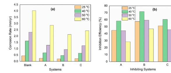
Fig. 22 Plots of (a) corrosion rate and (b) inhibition efficiency for X60 steel in 5% HCl without and with (A) 0.5% of CHT0.5–CuO, (B) CHT1.0–CuO, and (C) CHT2.0–CuO nanocomposites at different temperatures [reproduced from ref. 544, open access publication, copyright permission not required].
