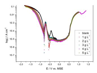
Fig. 30 Tafel plots obtained for AISI 304 stainless steel in 1.5 mol  $L^{-1}$   $H_2SO_4$  with and without the AW acid extract at a 1 mV s<sup>-1</sup> scanning rate<sup>626</sup> [reproduced for ref. 626, open access publication, copyright permission is not required].
