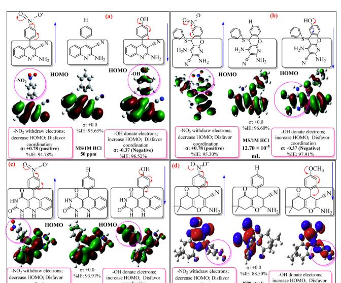
Fig. 7 Schematic illustration of the effect of some common substituents on the inhibition potential of some representative series of organic inhibitors. 11 [Reproduced from ref. 11 with permission, Copyright, Elsevier, 2023.]
