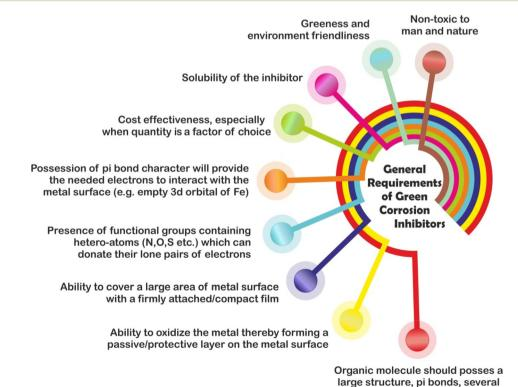
Fig. 4 Schematic illustration of the general requirements of a compound to be used as a corrosion inhibitor [self-illustration, copyright permission not required].
