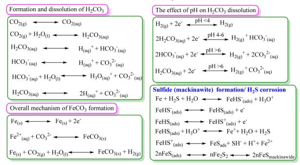
Fig. 6 Schematic presentation of the formation of H<sub>2</sub>CO<sub>3</sub> and FeCO<sub>3</sub> at different pH in CO<sub>2</sub>-rich (sweet) environment and mackinawite (nFeS) in H<sub>2</sub>S-rich (sour) environment [self-illustration, copyright permission not required].
