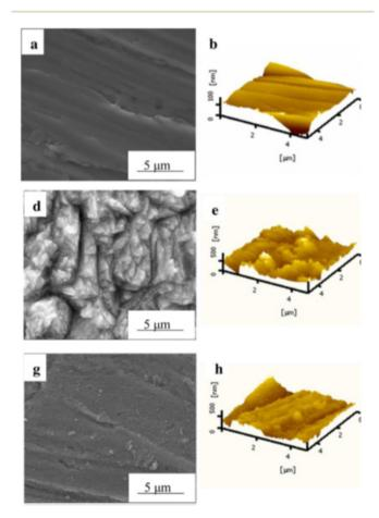
**Fig. 24** SEM (a, d, and g), AFM (b, e, and h), and contact angle images (c, f, and i) of CRS surfaces: (a–c) before immersion; (d–f) after 6 h of immersion at 20 °C in 1.0 M HCl solution; (g–i) after 6 h of immersion at 20 °C in 50 mg  $L^{-1}$  CS-SAS-AAGC + 1.0 M HCl solution [reproduced from ref. 583, open access publication, copyright permission is not required].
