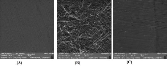
Fig. 31 SEM images of AISI 304 stainless steel: (A) before immersion, (B) after immersion in  $H_2SO_4$ , and (C) after immersion in  $H_2SO_4$  containing 5 g  $L^{-1}$  of AW acid extract (1500x increase). [reproduced for ref. 626, open access publication, copyright permission is not required].
