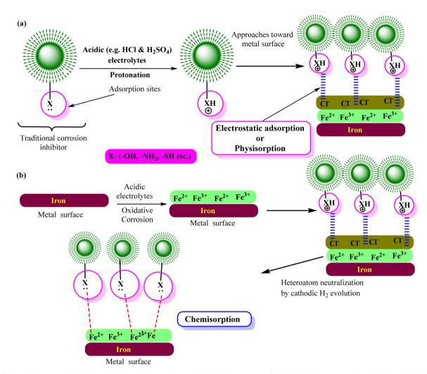
Fig. 5 Schematic presentation of the adsorption of a corrosion inhibitor having an amino  $(-NH_2)$  substituent on steel surface in acidic (HCl,  $H_2SO_4$ , etc.) and the mode of physisorption and chemisorption [self-illustration, copyright permission not required].
