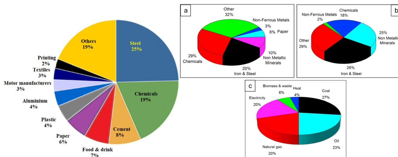
Fig. 8 (Left) Greenhouse gas (GHG) emissions from the UK industry.<sup>119</sup> [Reproduced from ref. 119 with permission, Copyright, Elsevier, 2021.] (Right) (a) Share of energy consumption in the industrial sector; (b)  $\text{CO}_2$  emissions and (c) final energy use in the industrial sector by fuel type.<sup>120</sup> [Reproduced from ref. 120 with permission, Copyright, Elsevier, 2021.]
