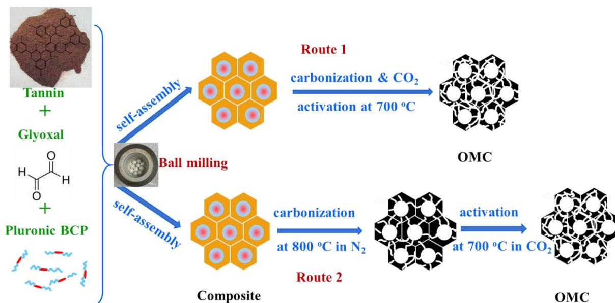
Fig. 14 Diagrammatic representation of the two processes used in the mechanochemical synthesis of OMCs: carbonization under  $\text{N}_2$  and subsequent  $\text{CO}_2$  activation (route 2); one-step carbonization and  $\text{CO}_2$  activation (route 1) utilizing tannin, glyoxal, and block copolymer<sup>327</sup> [reproduced from ref. 327; open access article, copyright permission is not required].
