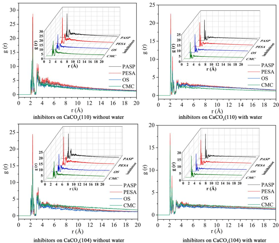
Fig. 29 Radial distribution function plot for the distance between the oxygen atom of inhibitors and the Ca-atom of calcite crystal surface<sup>601</sup> [reprinted with permission, Copyright, Elsevier, 2021].
