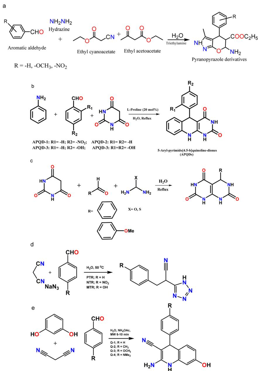
**Scheme 3** Scheme for the synthesis of corrosion inhibitors based on (a) pyranopyrazoles,<sup>376</sup> (b) pyrimidoquinolines,<sup>377</sup> (c) pyrimidine derivatives,<sup>378</sup> (d) tetrazoles,<sup>379</sup> and (e) quinoline derivatives<sup>380</sup> in an aqueous medium [the synthetic schemes were reproduced and suitable copyright permissions have been obtained].
