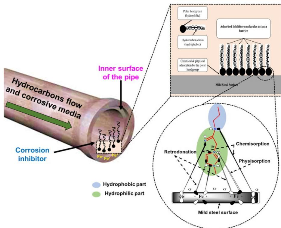
Fig. 34 Mechanism of action of Im-ILs in 1 M HCl<sup>662</sup> [reproduced from ref. 662 with permission, Copyright, Elsevier, 2023].
