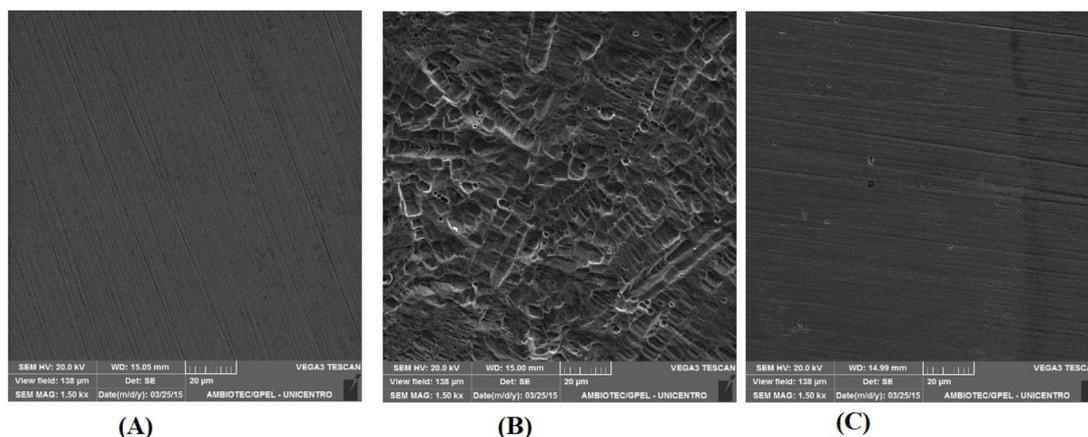
**Fig. 31** SEM images of AISI 304 stainless steel: (A) before immersion, (B) after immersion in  $\text{H}_2\text{SO}_4$ , and (C) after immersion in  $\text{H}_2\text{SO}_4$  containing  $5 \text{ g L}^{-1}$  of AW acid extract (1500X increase). [reproduced for ref. 626, open access publication, copyright permission is not required].
