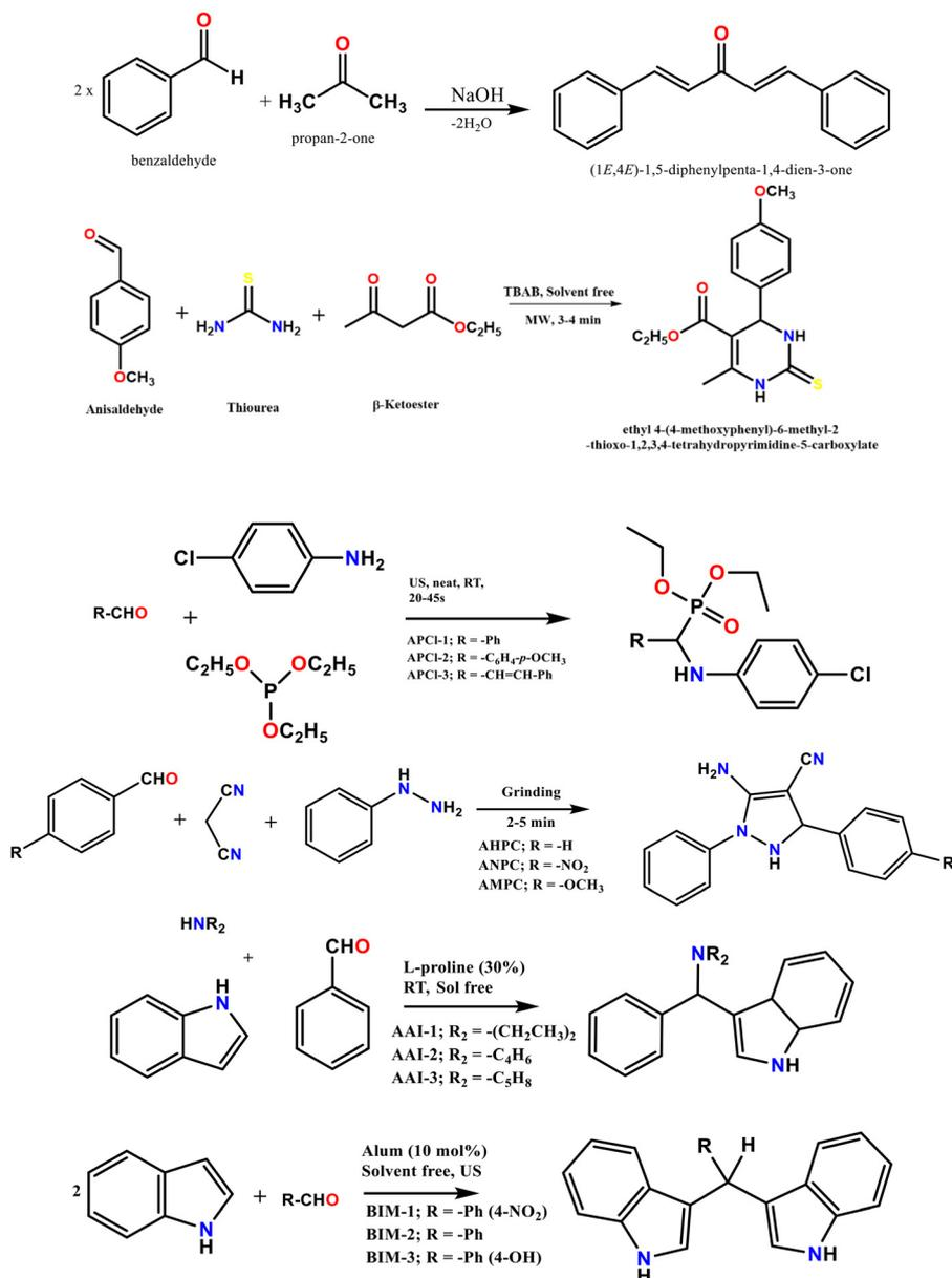
**Scheme 1** Solid-phase synthesis of (a) dibenzalacetone,<sup>343,344</sup> (b) pyrimidine derivatives,<sup>345</sup> (c) phosphonates,<sup>346</sup> (d) pyrazoles,<sup>324</sup> (e) 3-amino alkylated indoles,<sup>347</sup> and (f) bis(indolyl) methanes<sup>348</sup> [the synthetic schemes were reproduced and suitable copyright permissions have been obtained].
