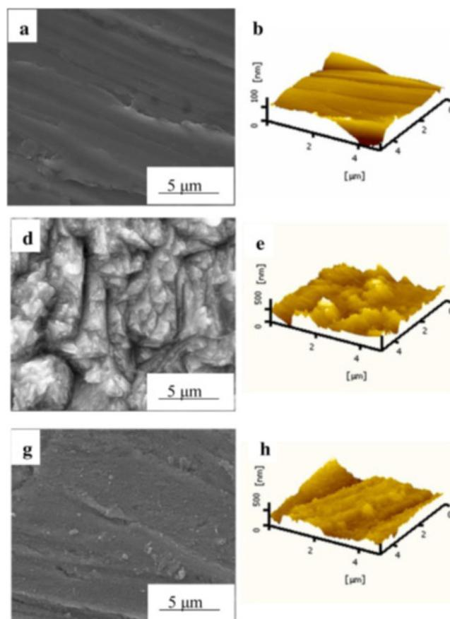
**Fig. 24** SEM (a, d, and g), AFM (b, e, and h), and contact angle images (c, f, and i) of CRS surfaces: (a–c) before immersion; (d–f) after 6 h of immersion at 20 °C in 1.0 M HCl solution; (g–i) after 6 h of immersion at 20 °C in 50 mg L<sup>-1</sup> CS-SAS-AAGC + 1.0 M HCl solution [reproduced from ref. 583, open access publication, copyright permission is not required].
