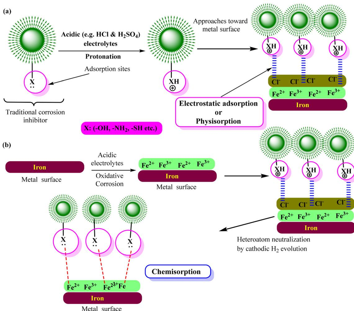
**Fig. 5** Schematic presentation of the adsorption of a corrosion inhibitor having an amino (–NH<sub>2</sub>) substituent on steel surface in acidic (HCl, H<sub>2</sub>SO<sub>4</sub>, etc.) and the mode of physisorption and chemisorption [self-illustration, copyright permission not required].
