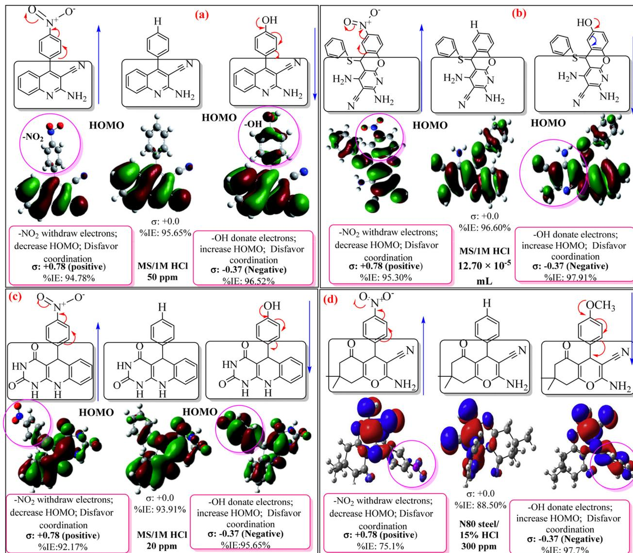
Fig. 7 Schematic illustration of the effect of some common substituents on the inhibition potential of some representative series of organic inhibitors.<sup>11</sup> [Reproduced from ref. 11 with permission, Copyright, Elsevier, 2023.]
