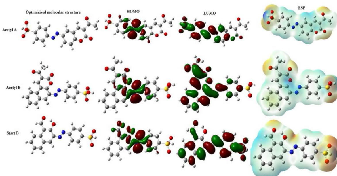
Fig. 35 Optimized, HOMO, LUMO, and ESP representations of the tested dyes as corrosion inhibitors<sup>730</sup> [reproduced from ref. 730, with permission, Copyright, Elsevier, 2022].
