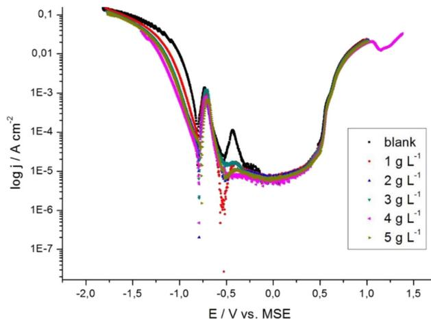
**Fig. 30** Tafel plots obtained for AISI 304 stainless steel in  $1.5 \text{ mol L}^{-1}$   $\text{H}_2\text{SO}_4$  with and without the AW acid extract at a  $1 \text{ mV s}^{-1}$  scanning rate<sup>626</sup> [reproduced for ref. 626, open access publication, copyright permission is not required].
