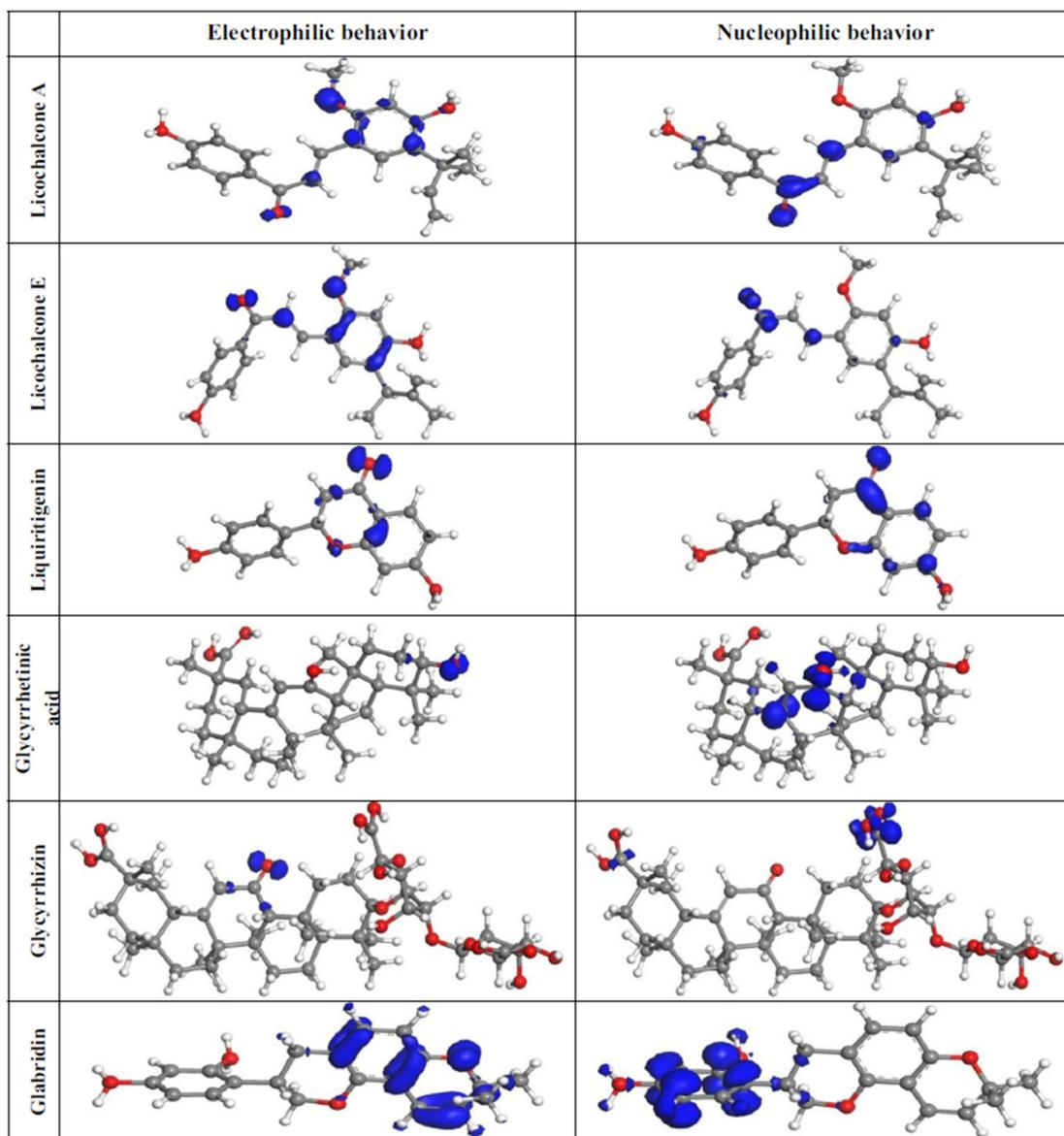
Fig. 27 Fukui index calculation for protonated licochalcone A, licochalcone E, liquiritigenin, 18 $\beta$ -glycyrrhetic acid, glycyrrhizin, and glabridin present in *Glycyrrhiza glabra* leaf extract<sup>594</sup> [reproduced from ref. 594 with permission, Copyright, Elsevier, 2018].
