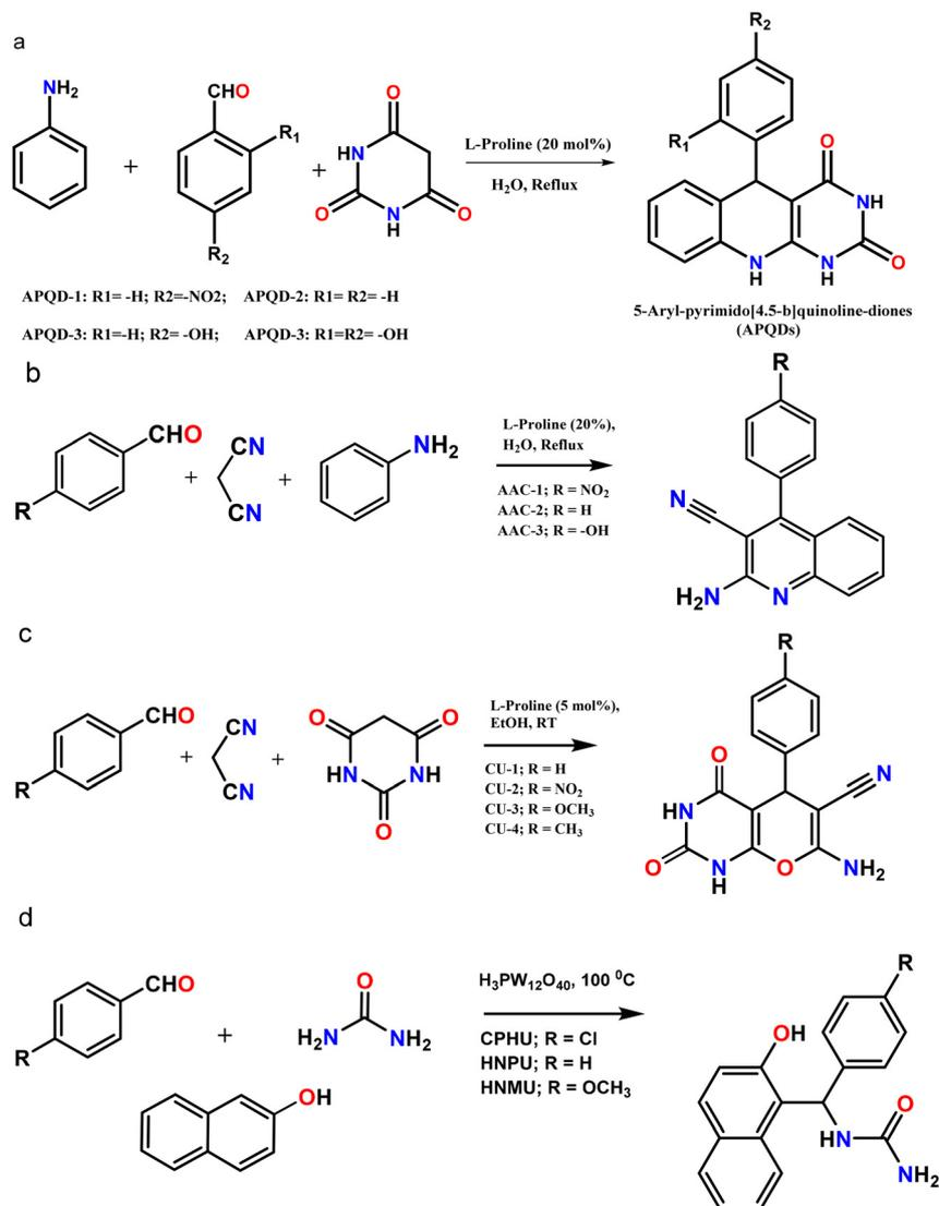
**Scheme 5** Schemes for the synthesis of corrosion inhibitors based on (a) pyrimidoquinolines,<sup>403,404</sup> (b) quinoline derivatives,<sup>405</sup> (c) condensed uracils,<sup>406</sup> and (d) urea derivatives<sup>407</sup> using environmentally safer catalysts [the synthetic schemes were reproduced and suitable copyright permissions have been obtained].
