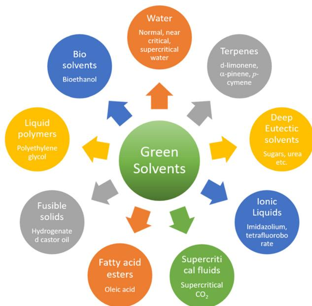
**Fig. 18** Different types of green solvents [self-illustration, copyright permission is not required].
