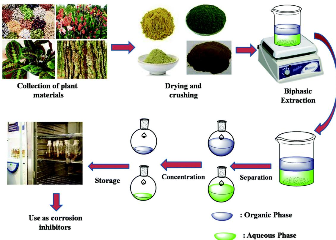
Fig. 11 Schematic diagram of extraction procedure of phytochemicals.<sup>20</sup> [Reproduced from ref. 20, RSC publication, copyright permission is required.]
