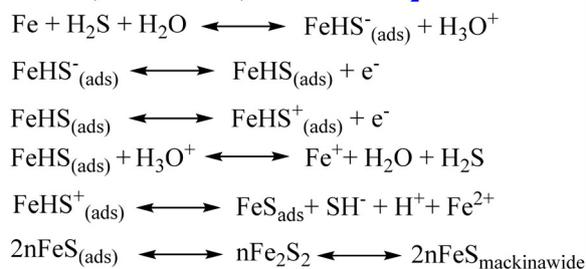
**Fig. 6** Schematic presentation of the formation of H<sub>2</sub>CO<sub>3</sub> and FeCO<sub>3</sub> at different pH in CO<sub>2</sub>-rich (sweet) environment and mackinawite (nFeS) in H<sub>2</sub>S-rich (sour) environment [self-illustration, copyright permission not required].
