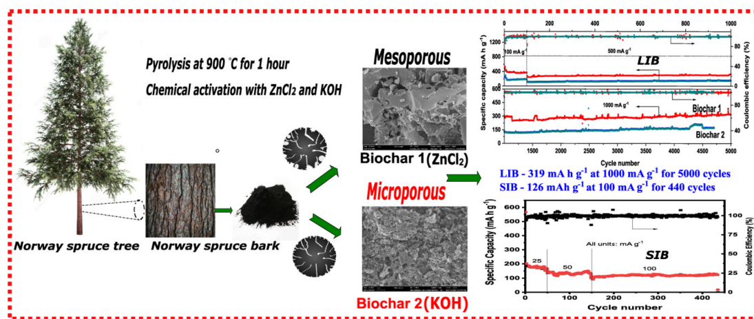
Fig. 2 Synthesis of carbon anodes prepared using different chemical activation with \text{ZnCl}_2 (Biochar-1) and \text{KOH} (Biochar-2) and tested in LIBs and SIBs. Reproduced with permission. 41 Copyright 2022, American Chemical Society.
