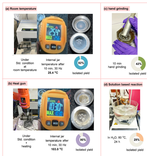
Fig. 2 Various reaction setups: (a) reaction at room temperature; (b) heat gun-based reaction; (c) hand grinding-based reaction; (d) solution-based reaction.
