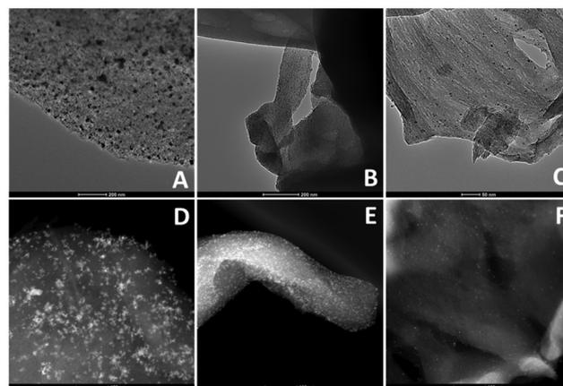
Fig. 6 HRTEM (A, B and C) and STEM (D, E and F) micrographs of the Rh-N/C samples with 5%, 3% and 1% of Rh respectively.
