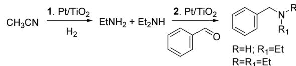
**Scheme 2** Pt/TiO<sub>2</sub> nanocatalyst for a cascade reaction: 1: hydrogenation of acetonitrile; 2: reductive amination of benzaldehyde.
