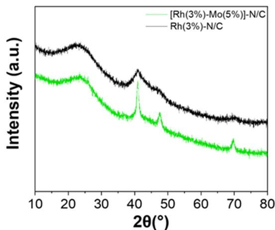
Fig. 8 XRD patterns of the sample [Rh(3%)-Mo(5%)]-N/C (green) compared with the monometallic sample Rh(3%)-N/C (black).
