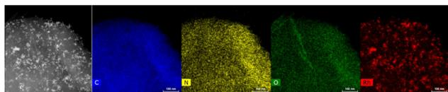
Fig. 18 HRTEM in STEM mode-EDX micrographics of the Rh(5%)-N/C used sample.
