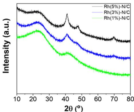
Fig. 2 XRD patterns of the Rh-based materials with loading of 5 wt% (black), 3 wt% (blue), and 1 wt% (green).
