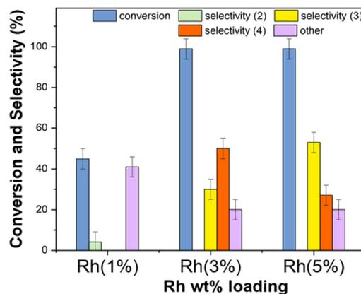
**Fig. 13** Reductive amination of benzaldehyde with ACN (10 mL) carried out at 100 °C, 30 bar of H<sub>2</sub>, and 24 h. Catalysts (50 mg) were mono-metallic Rh-based systems with 1, 3, and 5 wt% metal loading. The colored bars refer to conversion (blue), and amounts of products, 2 (green), 3 (yellow), 4 (orange), and others (violet).
