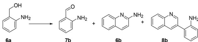
**Scheme 9** The reaction of 2-aminobenzyl alcohol (**6a**) under oxidative conditions (170 °C; 1 atm, 18 h,  $V_{ACN} = 10$  mL). 2-aminobenzyl aldehyde iminoquinoline (**6b**), and 2-(3-quinolinyl) aniline (**8b**) were the observed products.
