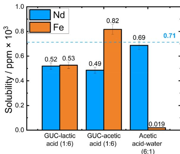
**Fig. 5** Dissolution of  $Nd_2O_3$  and  $Fe_2O_3$  with ratio of 1:7 wt% ratio in 1.5 mL of GUC–lactic acid and GUC–acetic acid with molar ratio of 1:6, acetic acid–water (6:1) at 50 °C for 24 h. Blue line indicates the initial concentration of Nd ( $0.71 \times 10^3$  ppm) used for the leaching experiments. The initial concentration of Fe was  $3.92 \times 10^3$  ppm, and therefore not included in the graph for increased clarity.
