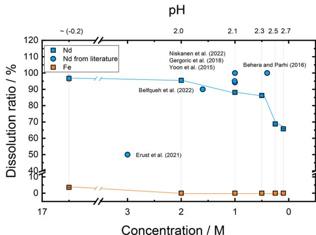
**Fig. 6** Dissolution efficiency of Nd and Fe from the mixture of  $\text{Nd}_2\text{O}_3$  and  $\text{Fe}_2\text{O}_3$  (13 wt%–87 wt%) using acetic acid with different concentrations at 50 °C for 24 h. Blue and orange squares indicate Nd and Fe dissolution ratios in this work. Blue circles indicate Nd dissolution ratio from the literature.
