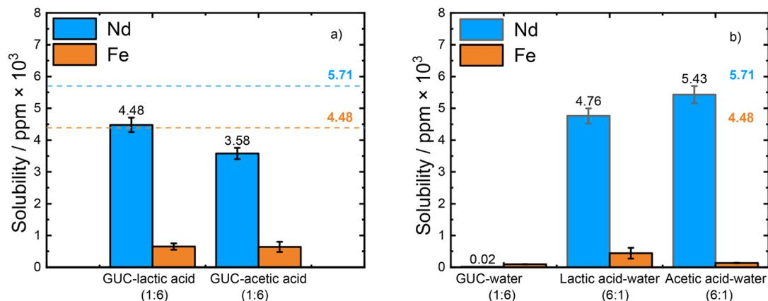
**Fig. 1** Dissolution of 10 mg  $\text{Nd}_2\text{O}_3$  or  $\text{Fe}_2\text{O}_3$  in 1.5 mL of reagents composed of (a) HBAs and HBDs with the molar ratio of (1 : 6), (b) HBA and water (1 : 6); and HBDs and water (6 : 1) at 50 °C for 24 h. Blue and orange dashed lines indicate the initial concentration of Nd ( $5.71 \times 10^3$  ppm) and Fe ( $4.48 \times 10^3$  ppm) oxides, respectively, before the leaching experiments.
