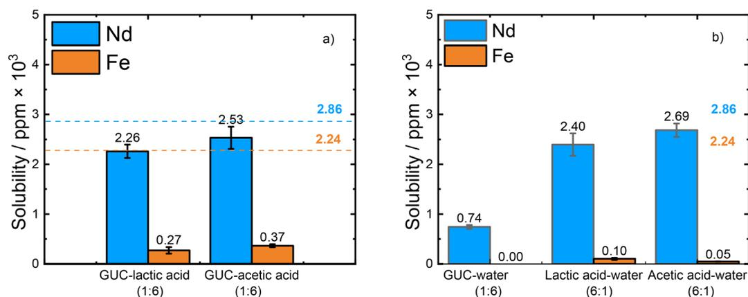
Fig. 3 Dissolution of  $\text{Nd}_2\text{O}_3$  (5 mg) and  $\text{Fe}_2\text{O}_3$  (5 mg) with a 1 : 1 wt ratio in 1.5 mL of solvents composed of (a) HBAs and HBDs with the molar ratio of 1 : 6, (b) HBA and water (1 : 6) and HBDs and water (6 : 1) at 50 °C for 24 h. Blue and orange dashed lines indicate the initial concentration of Nd ( $2.86 \times 10^3$  ppm) and Fe ( $2.24 \times 10^3$  ppm) used for the leaching experiments.
