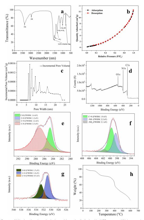
Fig. 3 (a) FT-IR spectra; (b) N<sub>2</sub> adsorption-desorption isotherms; (c) pore size distribution; (d-g) XPS spectra; and (h) thermogravimetric analysis of the MFR.
