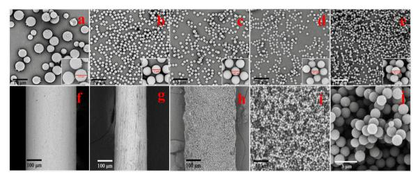
Fig. 2 SEM images of the MFRs (a—e) with a PVP quality of 0, 0.10, 0.30, 0.50, and 0.70 g, respectively. SEM images of the fiber (f) before and (g) after corroding by using aqua regia; SEM images of the MFR-based SPME fiber at different magnifications: (h) ×500; (i) ×25000.
