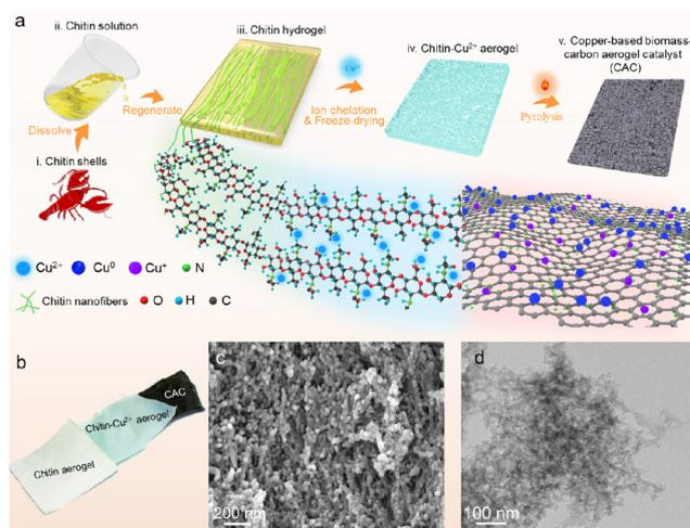
**Fig. 2** (a) Schematic diagram of the preparation of the copper-based biomass carbon aerogel catalyst (Cu(OTf)<sub>2</sub>@CAC). (b) Photographs of chitin aerogels, chitin/Cu<sup>2+</sup> composite aerogels, and aerogel catalysts. (c) SEM image of Cu(OTf)<sub>2</sub>@CAC. (d) High magnification TEM image of Cu(OTf)<sub>2</sub>@CAC.
