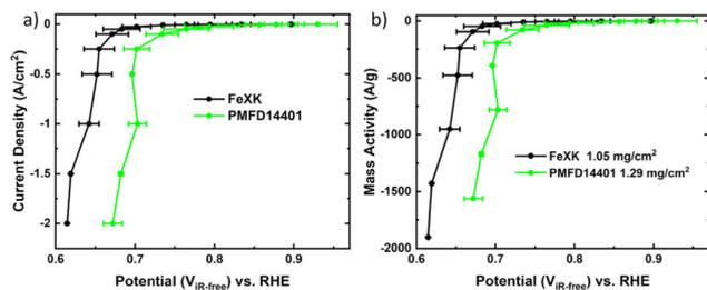
**Fig. 6** GDE measurement in cathodic direction of FeXK and PMFD14401 (loading 1.05 mg cm<sup>-2</sup> and 1.29 mg cm<sup>-2</sup> respectively) in KOH 1 M (a) iR-corrected for electrolyte resistance (100% post correction from phase angle closest to 0 in high-frequency region >1000 Hz). (b) and after normalization to catalyst loading. Error bars represent two repeat measurements.
