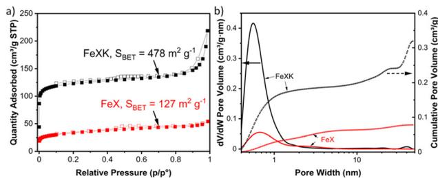
Fig. 2  $N_2$  sorption isotherms, where solid and empty squares indicate adsorption and desorption isotherms (a). Pore size distributions and cumulative pore volumes determined using the 2D-NLDFT heterogeneous surface carbon model within SAIEUS software (b). Data for FeX and FeXK.
