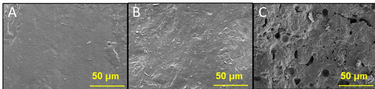
Fig. 4 Scanning electron microscopy of untreated, granulate PET (A), leftover PET samples from hot compressed H<sub>2</sub>O (*i.e.* N<sub>2</sub>-H<sub>2</sub>O, with 208 psi of initial N<sub>2</sub> pressure) reaction (B), and CO<sub>2</sub>-H<sub>2</sub>O reaction (208 psi of initial CO<sub>2</sub> pressure) (C) at 165 °C (non-isothermal conditions). Reaction conditions: PET to H<sub>2</sub>O ratio 1 : 8 w/w (2.5 g PET : 20 mL H<sub>2</sub>O).
