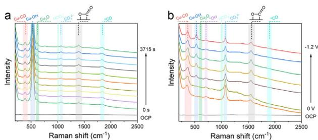
**Fig. 4** *In situ* Raman spectra of (a) the Cu<sub>100</sub>Al<sub>7.88</sub>-OD electrode at  $-1.68$  V vs. RHE with different reaction times during the eCO<sub>2</sub>RR in a 0.5 M KOH electrolyte and (b) the Cu<sub>100</sub>Al<sub>7.88</sub>-OD electrode at various potentials during the eCO<sub>2</sub>RR in a 0.5 M KOH electrolyte. All potentials are given vs. RHE.
