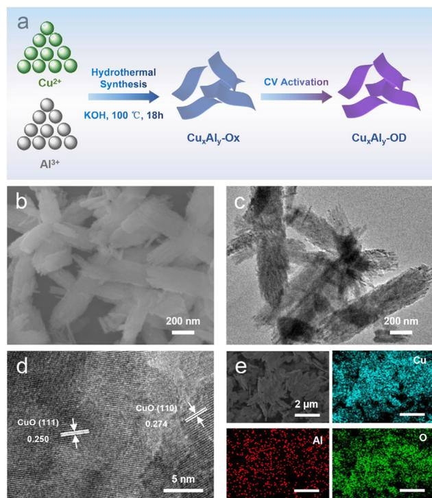
**Fig. 1** Preparation and characterization of catalysts. (a) Schematic illustration of the process to prepare  $\text{Cu}_x\text{Al}_y\text{-Ox}$  catalysts. (b) SEM, (c) TEM, (d) HRTEM, and (e) EDS elemental mapping images of the  $\text{Cu}_{100}\text{Al}_{7.88}\text{-Ox}$  catalyst.
