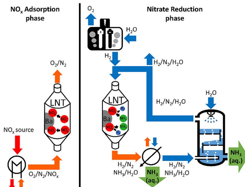
**Fig. 1** NOCCRA process. NO<sub>x</sub> adsorption phase: NO<sub>x</sub>-containing exhaust gas is cooled and sent over the LNT, which captures NO<sub>x</sub> on the Ba sites; nitrate reduction phase: H<sub>2</sub> generated through water electrolysis is sent over the LNT, reducing the captured NO<sub>x</sub> to NH<sub>3</sub> which is separated from the gas stream in a gas washing column.
