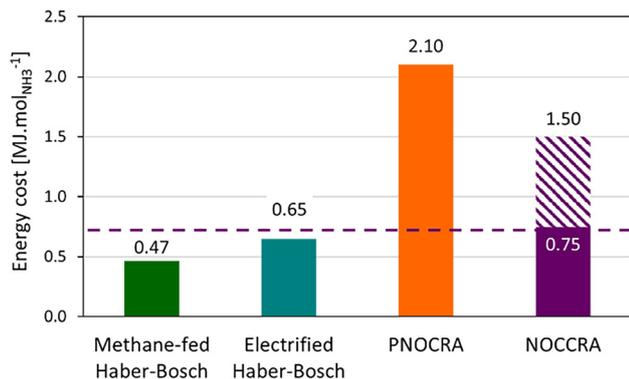
**Fig. 3** Energy requirement [MJ mol<sub>NH<sub>3</sub></sub><sup>-1</sup>] of the ammonia synthesis processes: natural gas-based Haber–Bosch,<sup>2</sup> electrified Haber–Bosch,<sup>2</sup> PNO CRA<sup>31</sup> and NOCCRA with and without accounting for the savings of NH<sub>3</sub> by avoiding the need for an S(N)CR process for NO<sub>x</sub> abatement.
