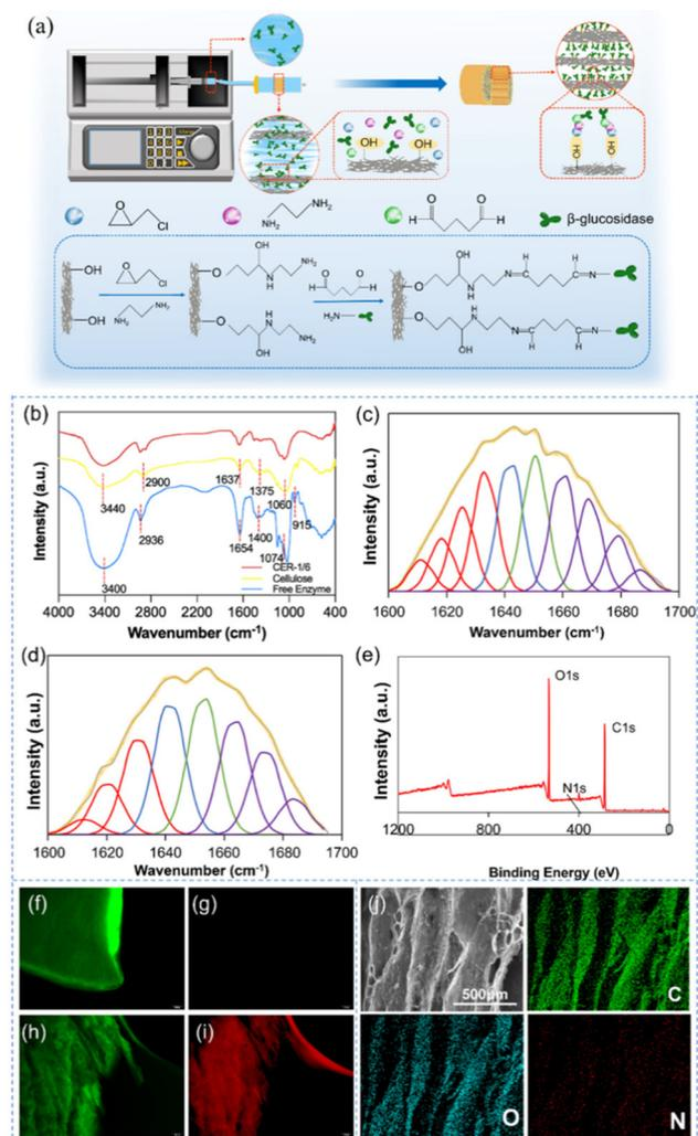
**Fig. 3** (a) Immobilized enzyme process; (b) FT-IR spectra of different materials; infrared deconvolution maps of amide: (c) free enzyme; (d) CER-1/6; (e) X-ray photoelectron spectroscopy (XPS) spectrum analysis of CER-1/6; (f–g) CE-STs in green and red fluorescence; (h–i) CER-1/6 in green and red fluorescence; (j) EDS spectra of CER-1/6.
