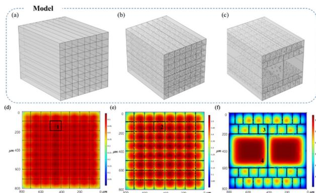
**Fig. 6** Models of reactors with different structures: (a) uniform nonporous channel; (b) uniform porous channel; (c) dual-scale channel; cloud diagram of substrate concentration changes: (d) uniform nonporous channel; (e) uniform porous channel; (f) dual-scale channel.
