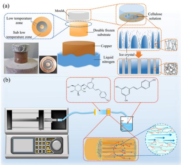
**Scheme 1** (a) Use of dual-scale ice crystal template constructing dual-scale directional channel structures; (b) construction of a dual-scale cellulose reactor and the formation of additional disturbances.
