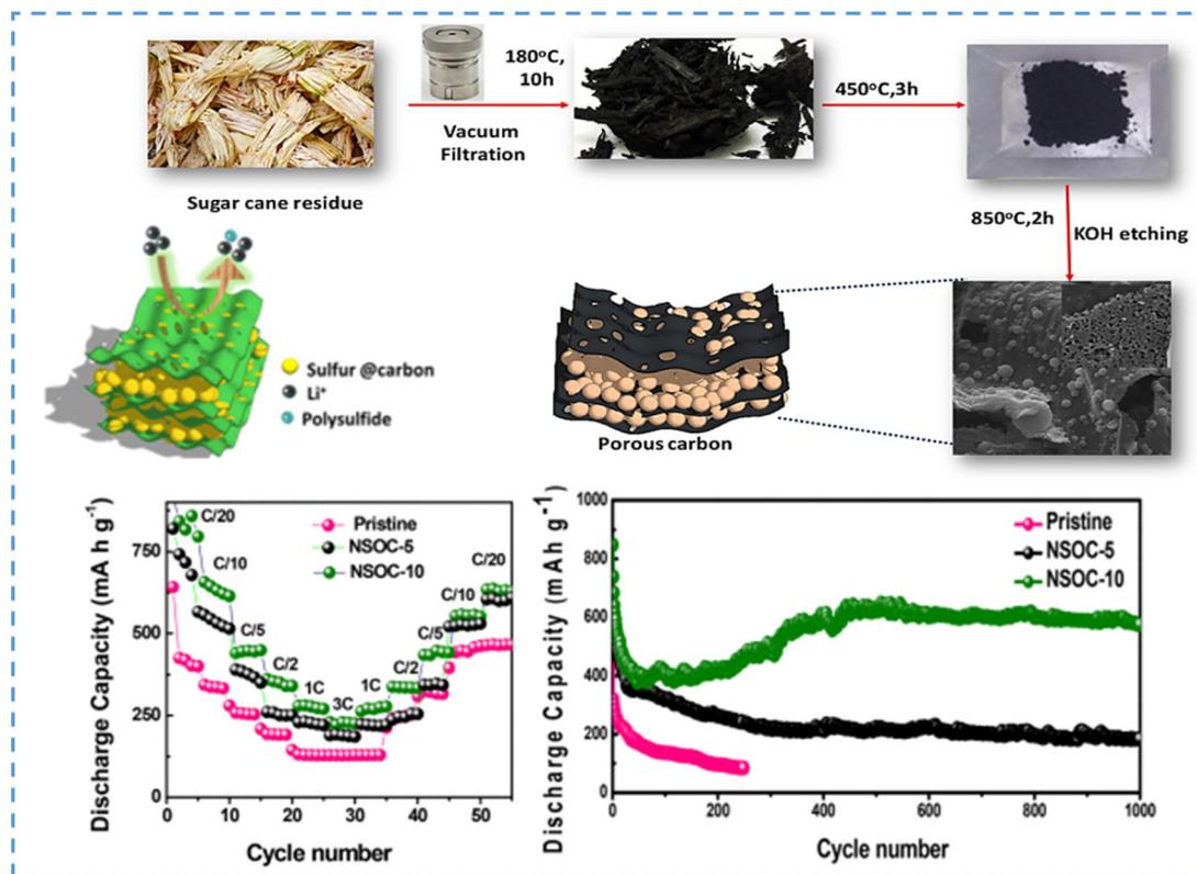
**Fig. 10** Schematic representation of the synthesis process for N, S, and O co-doped PC, discharge capacities at different rates, and cycling performance tests of pristine material, NSOC-5, and NSOC-10. Reproduced from ref. 321 with permission from American Chemical Society, copyright 2021.
