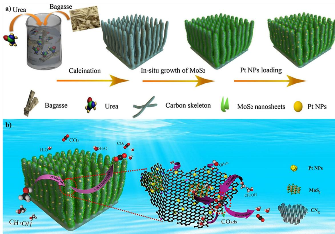
Fig. 6 Schematic representation of (a) the preparation of  $\text{Pt}/\text{MoS}_2/\text{CN}_x$  nanocomposites and (b) MOR using the  $\text{Pt}/\text{MoS}_2/\text{CN}_x$  catalyst. Reproduced from ref. 187 with permission from Elsevier, copyright 2017.
