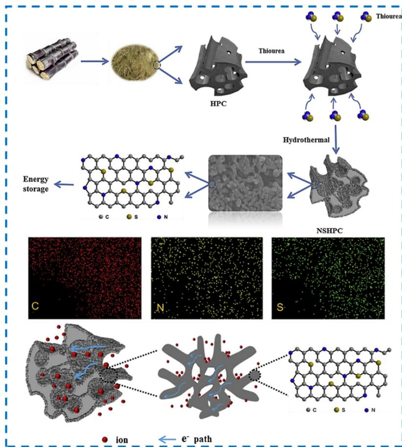
**Fig. 11** Schematic representation of the preparation process for the N–S doped hierarchical PC inherited from bagasse, EDS elemental mapping of doped hierarchical PC, and a schematic representation of transport paths for ions and electrons in the N–S doped hierarchical PC derived from bagasse. Reproduced from ref. 323 with permission from Elsevier, copyright 2019.
