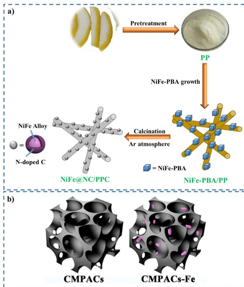
**Fig. 13** (a) Schematic representation of the preparation of NiFe@NC/PPC. Reproduced from ref. 332 with permission from Elsevier, copyright 2019. (b) Structures of the two kinds of electrodes (CMPACs and CMPACs-Fe). Reproduced from ref. 333 with permission from American Chemical Society, copyright 2018.
