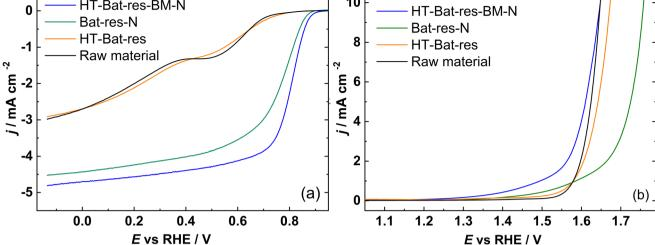
Fig. 3 RDE electrochemical characteristics of the studied materials: (a) ORR polarization curves at 1600 rpm in O2-saturated 0.1 M KOH solution and (b) OER polarization curves at 1600 rpm in N<sub>2</sub>-saturated 1 M KOH solution.
