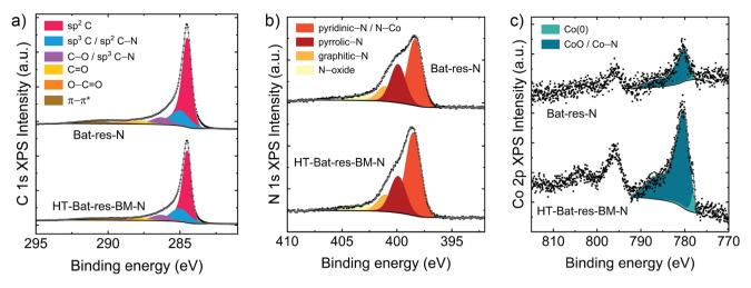
Fig. 2 X-ray photoelectron spectra of the Bat-res-N and HT-Bat-res-BM-N samples: (a) C 1s region, (b) N 1s region and (c) Co 2p region.
