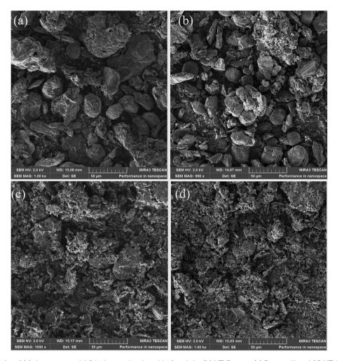
Fig. 1 SEM micrographs of (a) the raw material (black mass leach residue) and the (b) HT-Bat-res, (c) Bat-res-N and (d) HT-Bat-res-BM-N catalyst materials at 1000× magnification.
