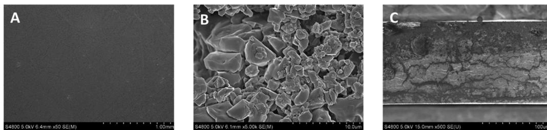
Fig. 6 SEM images of (A) the surface with a 1.00 mm scale bar, (B) the surface with a 10  $\mu\text{m}$  scale bar, and (C) the cross-section of L-WP films.
