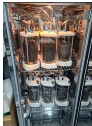
Fig. 2 Incubation chamber for the bioreactors of the ECHO analyzer system.
