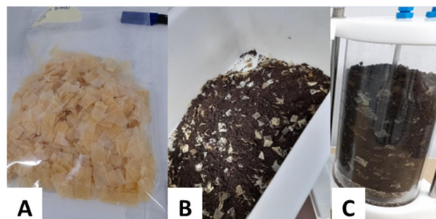
Fig. 1 Preparation of film samples for the biodegradation test: (A) film pieces, (B) mixture of film pieces and compost, and (C) one of the bioreactor vessels with the mixture of compost and film samples.
