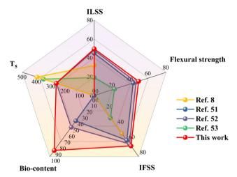
Fig. 5 Radar plot for qualitatively comparing five key aspects: ILSS, flexural strength, and IFSS for the composites, the thermal decomposition temperatures at 5% weight loss ( $T_5$ ), and bio-contents for the prepared sizing agents.
