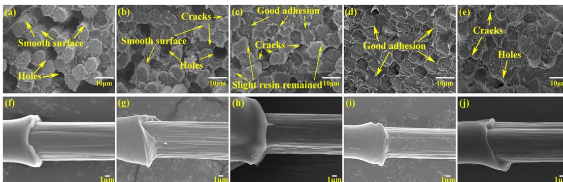
Fig. 6 SEM micrographs of the fracture morphologies of the composites after ILSS examination (a–e) and IFSS tests (f–j). CF-0 wt% (a and f), CF-0.5 wt% (b and g), CF-1.0 wt% (c and h), CF-1.5 wt% (d and i), and CF-2.0% (e and j).
