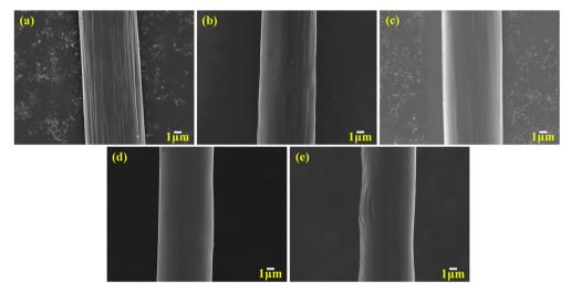
Fig. 3 SEM micrographs of CF surfaces subjected to varying concentrations of HWPU sizing agent: (a) unsized, (b) 0.5 wt%, (c) 1.0 wt%, (d) 1.5 wt%, and (e) 2.0 wt%.
