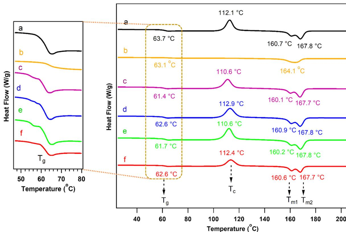
**Fig. 6** DSC thermograms (recorded during the second heating cycle) for neat PLA (a), PLA/Joncryl ADR (b), PLA/PCL-*g*-EAT 95/5 (c), PLA/PCL-*g*-EAT 90/10 (d), PLA/PCL-*g*-EAI 95/5 (e), and PLA/PCL-*g*-EAI 90/10 (f). Magnifications of the DSC graphs are provided at the left to show the  $T_g$  temperature.
