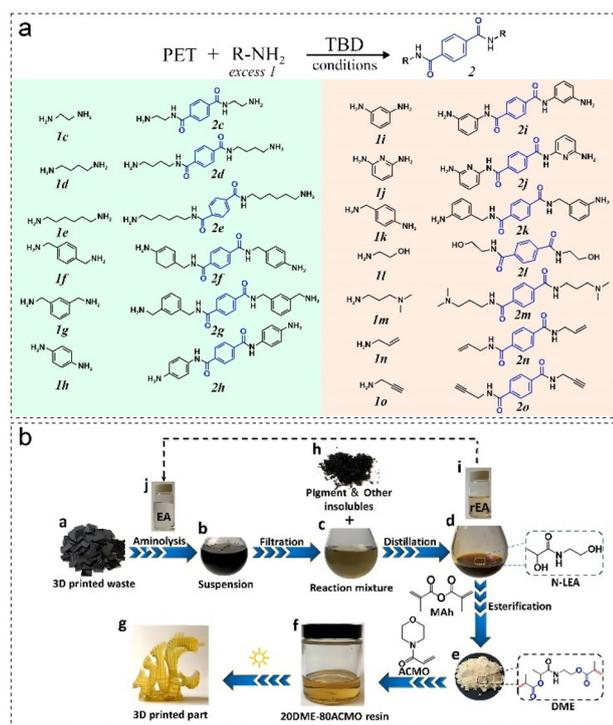
**Fig. 7** (a) Terephthalamides are produced through the organocatalytic aminolysis of PET,<sup>37</sup> and (b) schematic upcycling process from FDM 3D printed PLA waste to MSLA 3D printed photocurable resins.<sup>162</sup>
