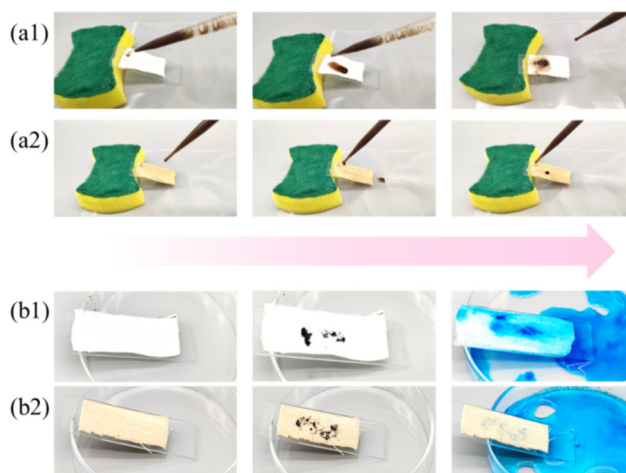
Fig. 10 Images of the anti-fouling performance of the (a1) pristine cotton fabric and (a2) FLP-50/Fe@cotton fabric. Self-cleaning performance of the (b1) pristine cotton fabric and (b2) FLP-50/Fe@cotton fabric.
