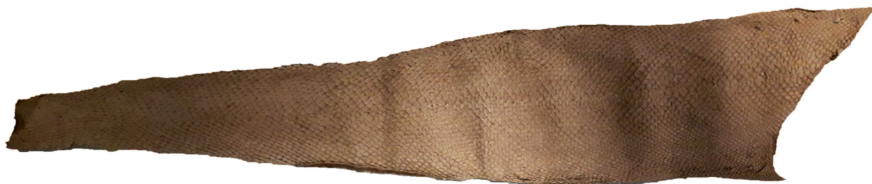
Fig. 1 Photo of salmon fish leather obtained by mimosa and chromium tanning.
