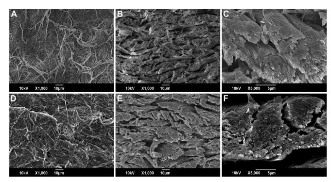
Fig. 4 (A-C) SEM image of the top view and cross-section of the untreated FL. (D-F) SEM image of the top view and cross-section of PESO 15.
