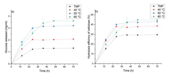
Fig. 3 (a) Glucose releasing rate and (b) hydrolysis efficiency of original and after one minute treatment with MSA-thymol at various temperature at different enzymatic hydrolysis times.
