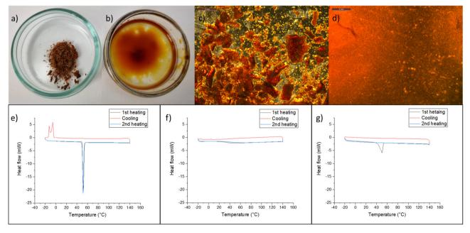
Fig. 4 Visual appearance of lignin and deep eutectic supramolecular polymer, and their thermal behavior (a and b) and isolated lignin (LF1) after heating with thymol at a mass ratio of 2:1 at 80 °C for 30 min (c and d) and differential scanning calorimetry curves of (e) thymol, (f) isolated lignin (LF1), and (g) a mixture of thymol and isolated lignin at a mass ratio of 2:1.
