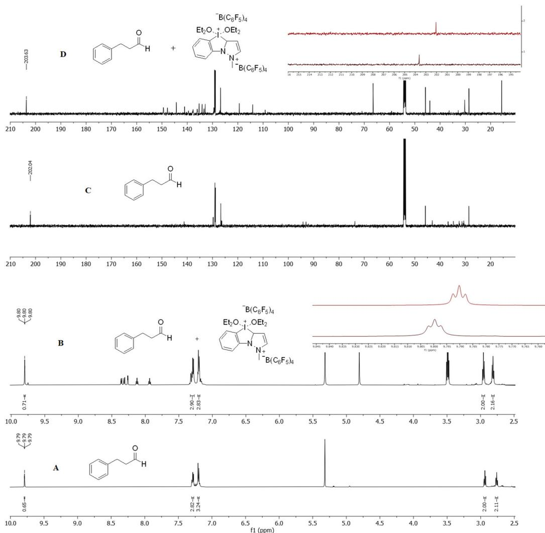
Fig. 2  $^1\text{H}$  NMR (600 MHz,  $\text{DMSO}-d_6$ ) studies of (A) 3-phenylpropanal (**1a**) and (B) the mixture of **1a** with **3e**, and  $^{13}\text{C}$  NMR (150 MHz,  $\text{DMSO}-d_6$ ) studies of (C) 3-phenylpropanal (**1a**) and (D) the mixture of **1a** with **3e**.
