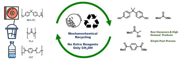
Fig. 1 Concept of mechanochemical recycling methanolysis of carbonate δ ester plastics: no catalyst, no solvent, and high efficiency.
