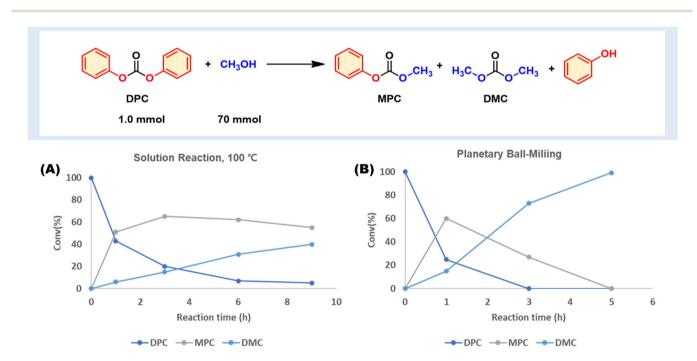
Fig. 2 Catalyst-free DPC methanolysis to DMC. (A) DPC and methanol mixture at 100 °C. (B) Planetary ball milling (SUS 12 mL, 5 mm balls 50 ea, 600 rpm).
