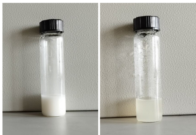
Fig. 7 The white precipitate observed in chitosan-[Cys][BF 4 ] as compared to the translucent solution in chitosan-[Ser][BF 4 ].
