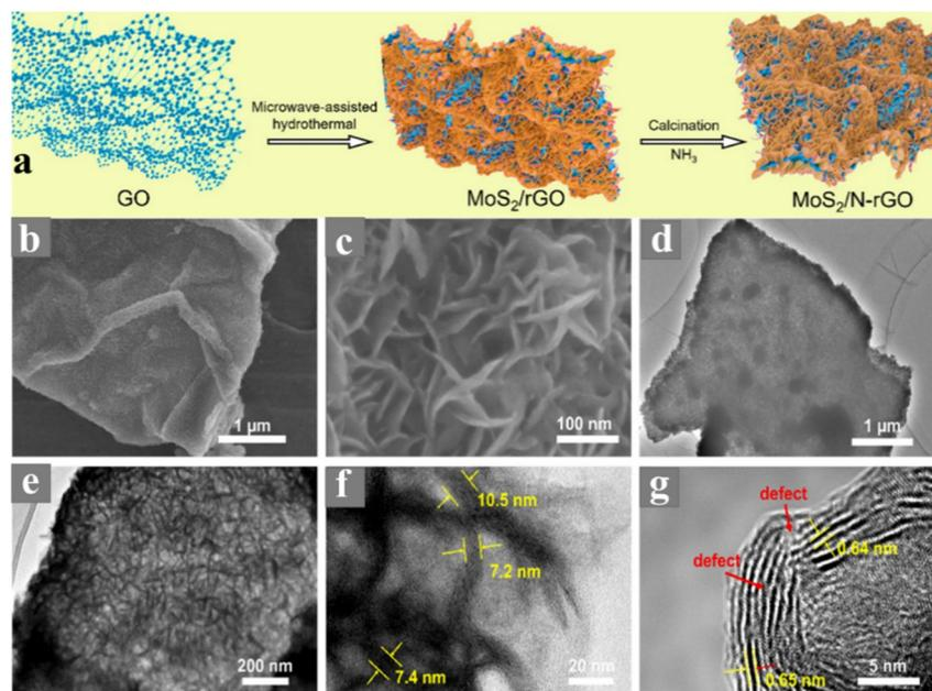
**Fig. 6** (a) Schematic reactions steps involved in the synthesis of MoS<sub>2</sub>/NGO vertical heterostructure, (b and c) SEM micrographs, (d and e) TEM micrographs, and (f and g) HRTEM images of MoS<sub>2</sub>/NGO vertical heterostructure. Reprinted with permission from ref. 82. Copyright 2021, Elsevier.
