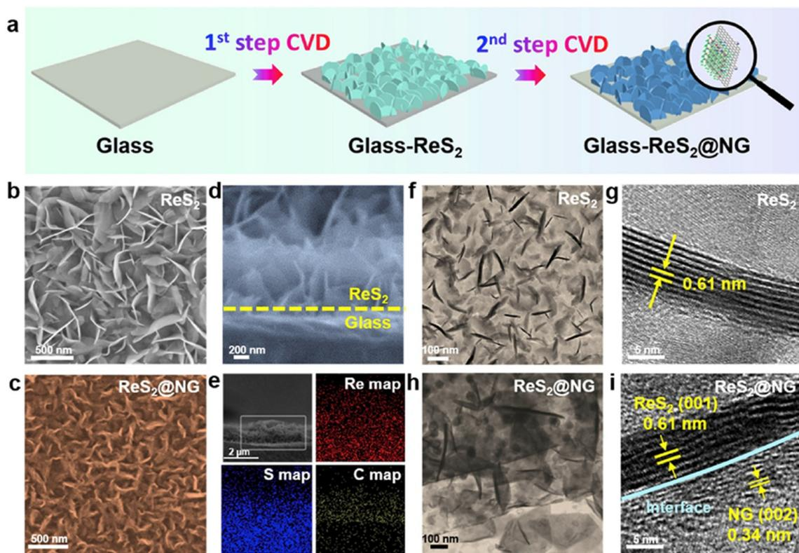
**Fig. 9** (a) Synthesis steps involved in the two-step CVD synthesis of  $\text{ReS}_2$ @NG, (b and c) SEM micrographs of  $\text{ReS}_2$  and  $\text{ReS}_2$ @NG nanosheets, (d and e) cross-sectional SEM micrograph of  $\text{ReS}_2$  nanosheets and  $\text{ReS}_2$ @NG nanosheets with corresponding elemental mapping, and (f–i) corresponding TEM and HRTEM micrographs of  $\text{ReS}_2$  and  $\text{ReS}_2$ @NG nanosheets. Reprinted with permission from ref. 87. Copyright 2019, Elsevier.
