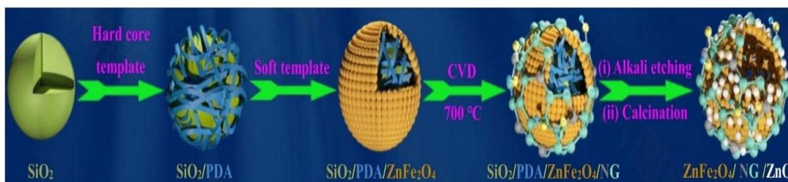
**Scheme 1** Reaction steps involved in the synthesis of ZnFe<sub>2</sub>O<sub>4</sub>/NG/ZnO heterostructure. Reprinted with permission from ref. 86. Copyright 2021, Elsevier.
