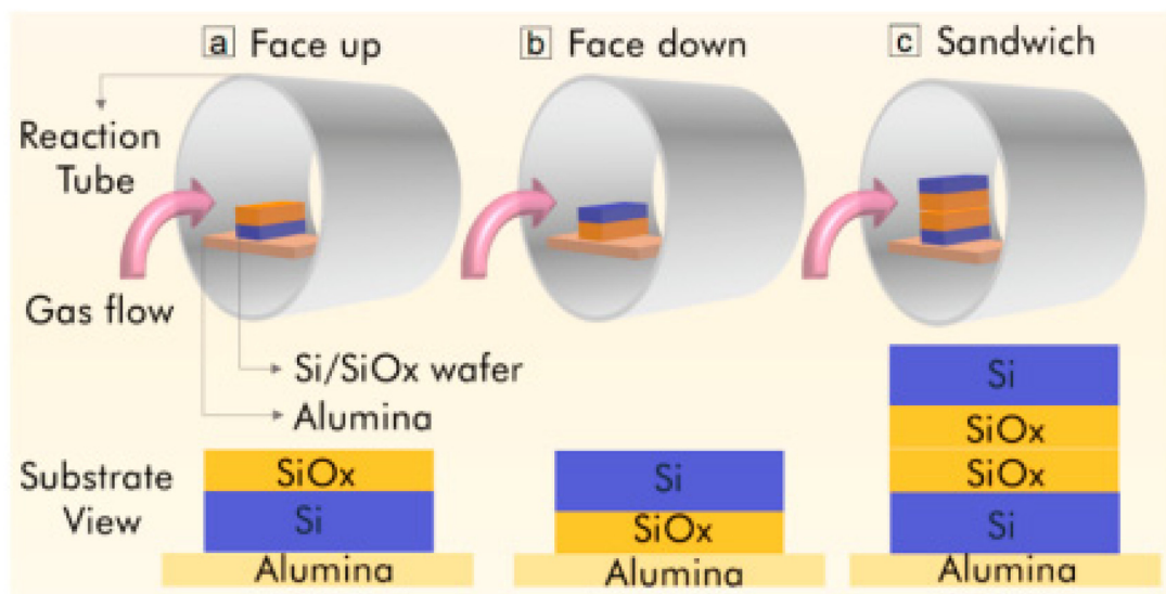
Fig. 13 (a) Schematic illustration of direct synthesis of graphene over Si/SiO x employing CVD approach with different configurations of substrate: (a) SiO x facing up, (b) SiO x facing down, and (c) Si/SiO x -SiO x /Si sandwiched configuration. Reprinted with permission from ref. 92. Copyright 2019, Wiley.
