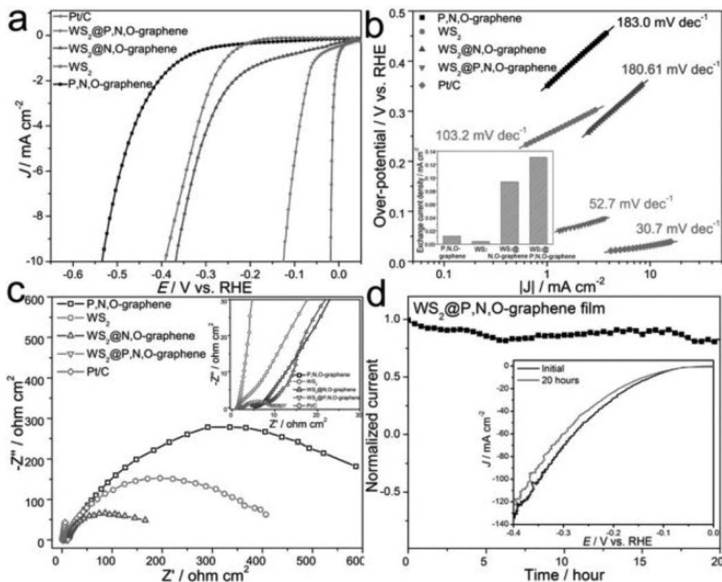
**Fig. 23** (a) LSV polarization curves below  $10 \text{ mA cm}^{-2}$ , (b) Tafel plots, (c) EIS spectra with enlarged spectra of as-prepared catalysts in inset, and (d) chronoamperometric response plot of  $\text{WS}_2@P,N,O$ -doped graphene film, with LSV polarization curves before and after 20 h of operation shown in inset. Reprinted with permission from ref. 203. Copyright 2017, Elsevier.
