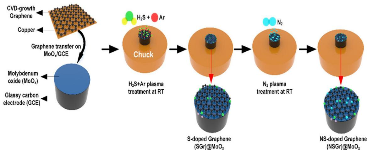
**Fig. 11** Schematic illustration of reaction steps used to synthesize NSGr@MoO<sub>x</sub> thin film heterostructure by ICP-assisted CVD approach. Reprinted with permission from ref. 90. Copyright 2023, Wiley.
