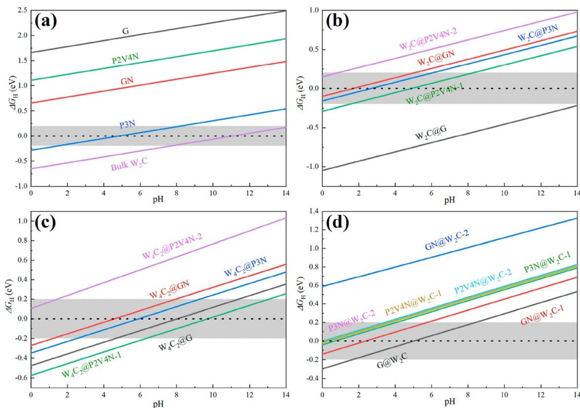
Fig. 27 pH-dependent H adsorption Gibbs free energy  $\Delta G_H$ . (a) Bulk  $W_2C$  and G-like models, (b)  $W_2C@G$ -like models, (c)  $W_4C_2@G$ -like models, and (d) G-like@ $W_2C$  models. Area in grey (HER preferable area)  $-0.1$  to  $0.2$  eV. Reprinted with permission from ref. 236. Copyright 2021, Elsevier.
