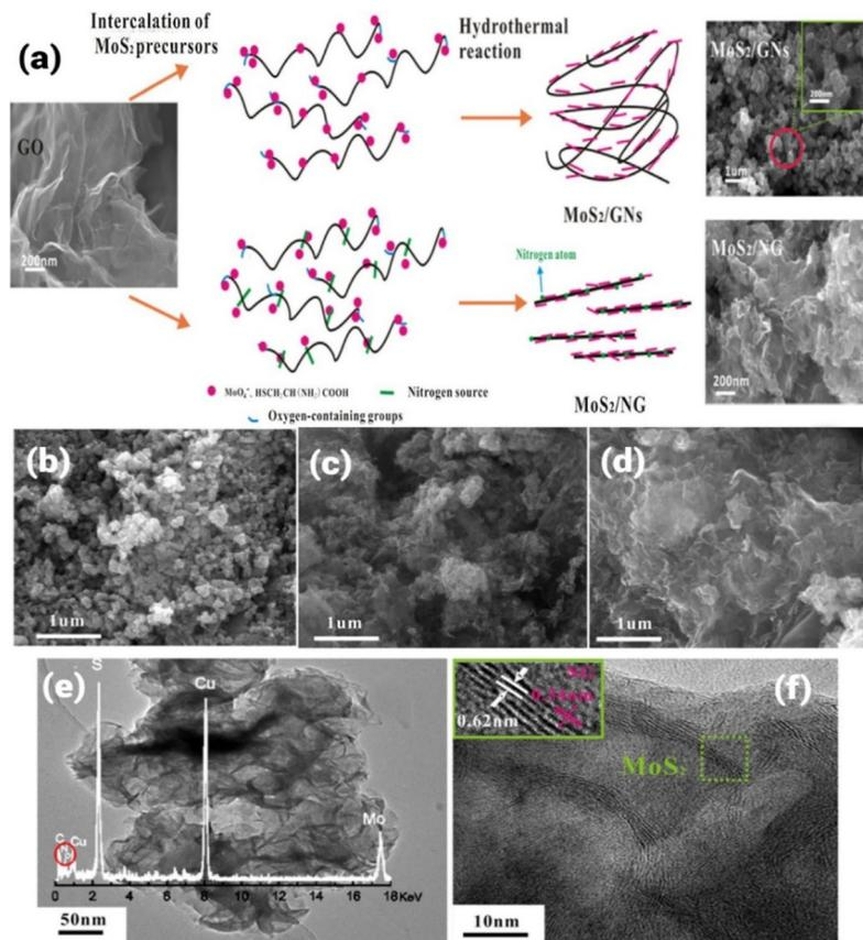
**Fig. 3** (a) Schematic representation of the synthesis of MoS<sub>2</sub>/NG and MoS<sub>2</sub>/graphene nanosheet hybrids using typical hydrothermal approach, (b–d) SEM micrographs at 1.5 : 1, 3 : 1 and 5 : 1 ratio of Na<sub>2</sub>MoO<sub>4</sub> : GO respectively, and (e) TEM and (f) HRTEM micrographs of MoS<sub>2</sub>/NG at 1.5 : 1 Na<sub>2</sub>MoO<sub>4</sub> : GO ratio. Reprinted with a permission from Reference (76). Copyright 2016, Elsevier.
