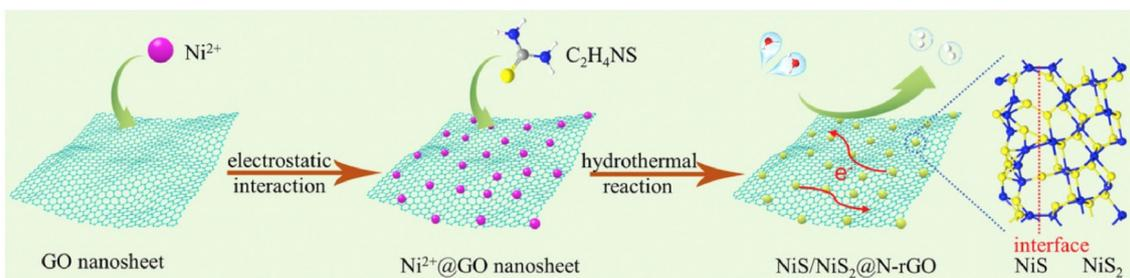
Fig. 5 Schematic reaction process for the synthesis of NiS/NiS<sub>2</sub>@N-rGO. Reprinted with permission from ref. 81. Copyright 2019, Elsevier.
