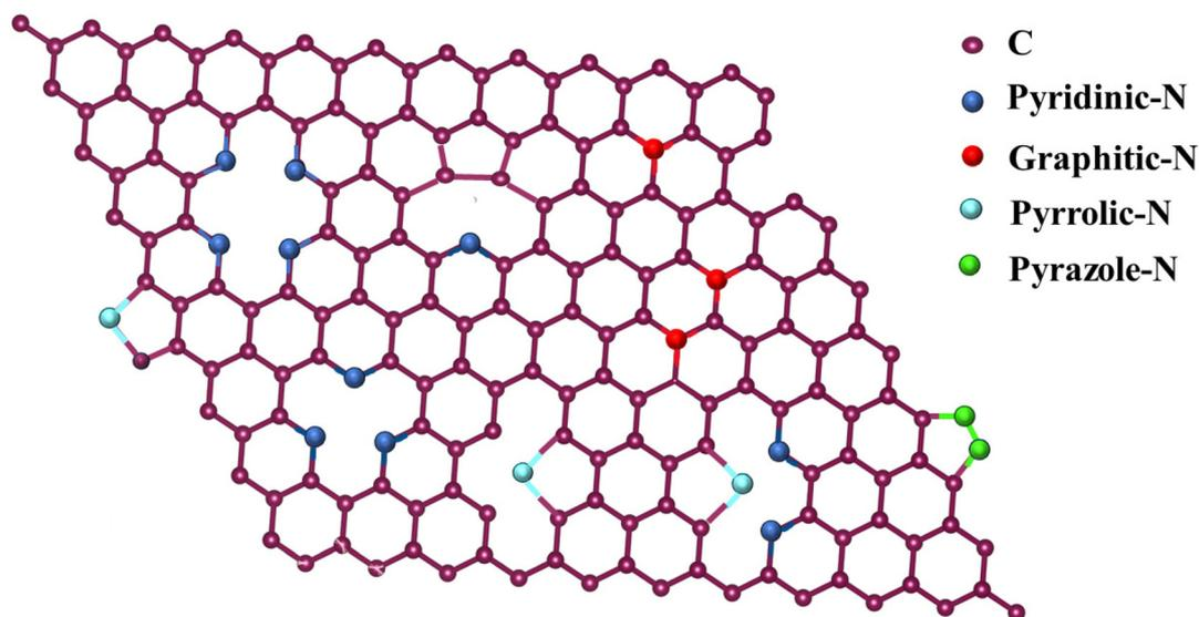
Fig. 16 Different configurations of N in nitrogen-doped graphene.
