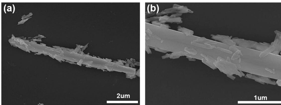
Fig. 4 (a and b) SEM micrographs of N-GQD/CdWO<sub>4</sub> at different scales. Reprinted with permission from ref. 78. Copyright 2017. Elsevier.
