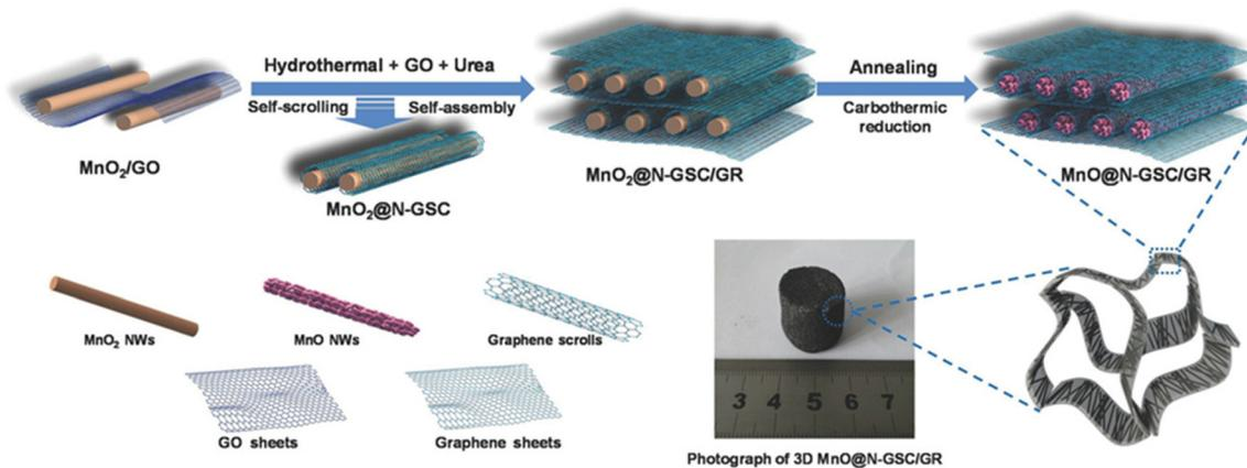
**Fig. 15** Schematic representation of the synthesis of hierarchical 3D MnO@NGS, which involves two steps, *i.e.*, self-scrolling and self-assembly process between GO sheets and MnO<sub>2</sub> nanowires, followed by annealing treatment. Reprinted with permission from ref. 98. Copyright 2017, Elsevier.
