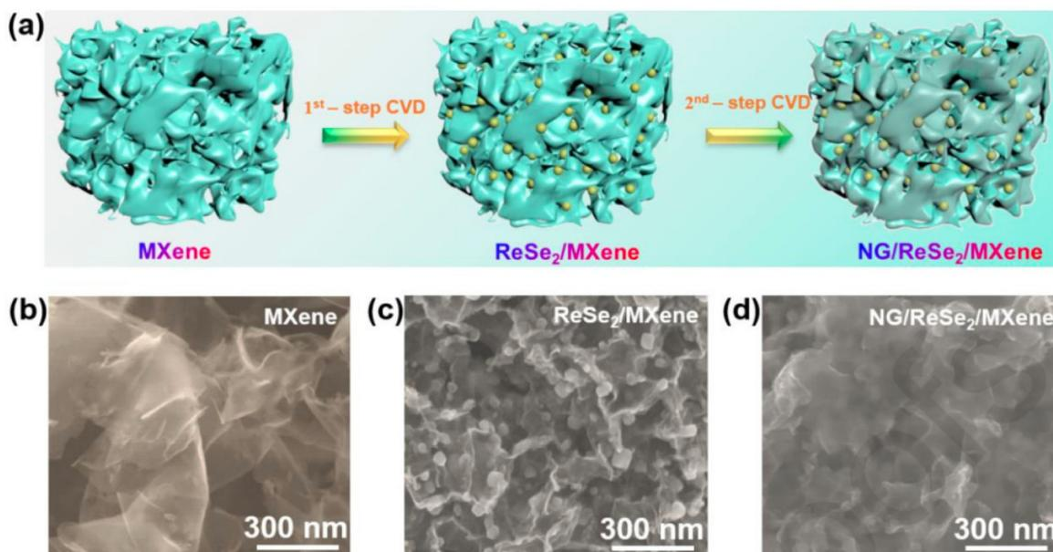
**Fig. 8** (a) Schematic illustration of CVD synthesis of NG/ReSe<sub>2</sub>/MXene and (b–d) SEM images of MXene, ReSe<sub>2</sub>/MXene and NG/ReSe<sub>2</sub>/MXene heterostructure, respectively. Reprinted with permission from ref. 84. Copyright 2015, Wiley.
