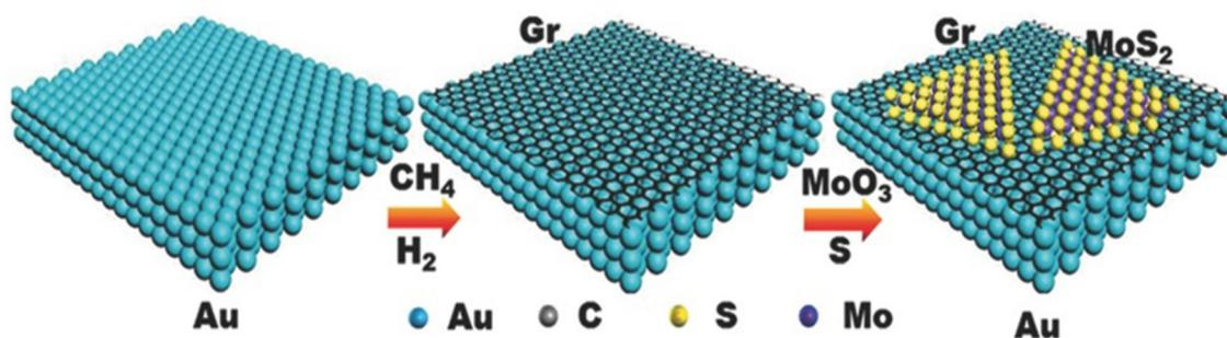
Fig. 7 Schematic illustration of reaction steps involved in the synthesis of MoS<sub>2</sub>/Gr heterostructure using CVD approach. Reprinted with permission from ref. 83. Copyright 2015, Wiley.
