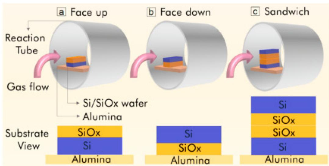
**Fig. 13** (a) Schematic illustration of direct synthesis of graphene over Si/SiO<sub>x</sub> employing CVD approach with different configurations of substrate: (a) SiO<sub>x</sub> facing up, (b) SiO<sub>x</sub> facing down, and (c) Si/SiO<sub>x</sub>-SiO<sub>x</sub>/Si sandwiched configuration. Reprinted with permission from ref. 92. Copyright 2019, Wiley.
