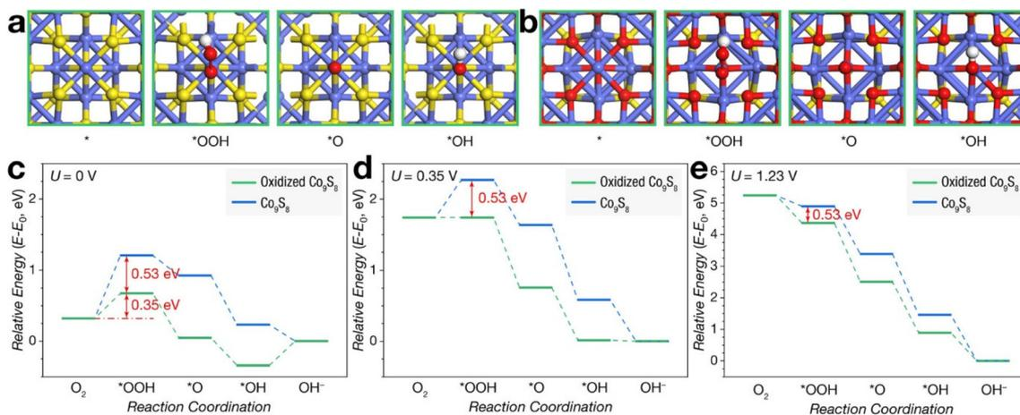
**Fig. 19** Optimised structure of intermediates adsorbed on (a and b) Co<sub>9</sub>S<sub>8</sub> and surface-oxidised Co<sub>9</sub>S<sub>8</sub> for ORR process and (c–e) energy landscapes calculated at  $U = 0$  V, 0.35 V and 1.23 V for Co<sub>9</sub>S<sub>8</sub> and surface-oxidised Co<sub>9</sub>S<sub>8</sub>, respectively. Reprinted with permission from ref. 173. Copyright 2020, the American Chemical Society.
