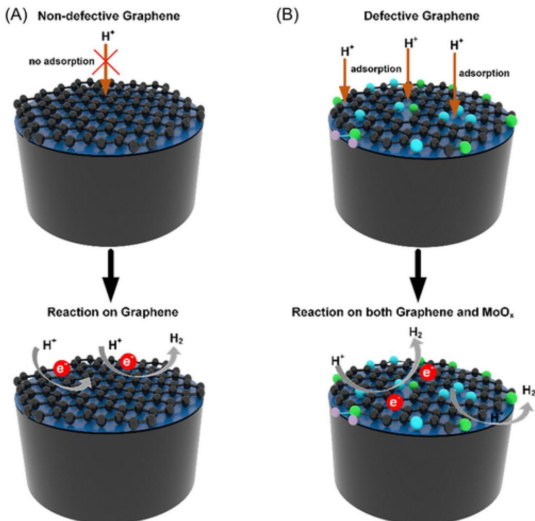
Fig. 22 Schematic illustration of the reaction steps involved in the HER over (A) undoped graphene and (B) N and S-co-doped graphene@MoO<sub>x</sub>/GCE hybrid electrode. Reprinted with permission from ref. 90. Copyright 2023, Wiley.
