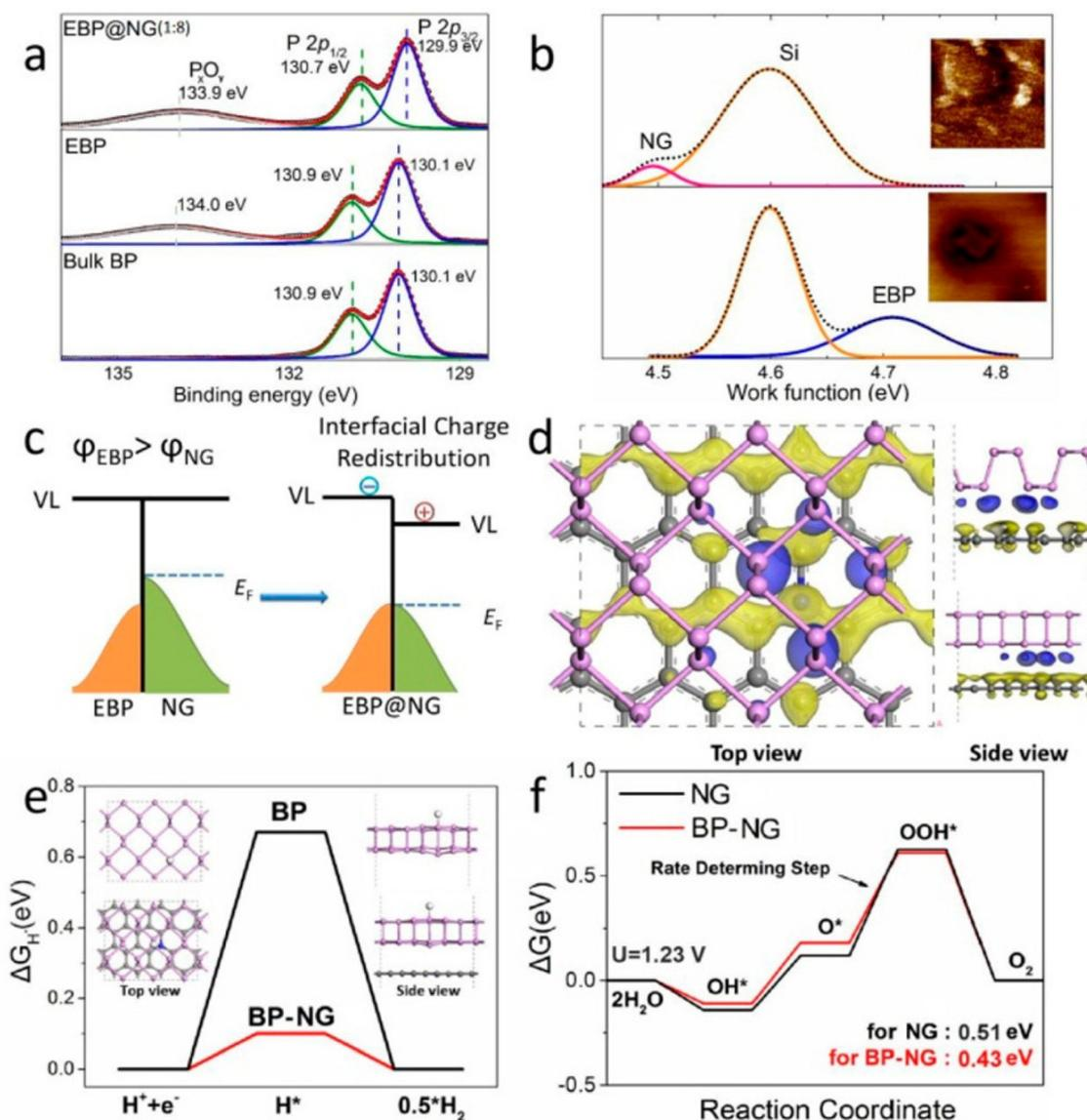
**Fig. 24** (a) P 2p XPS spectra of reference and EBP@NG samples, (b) work function plots of NG and EBP samples, (c) redistribution of interfacial charge between EBP and NG, (d) differential charge density of EBP and NG with yellow and blue for hole- and electron-rich area, respectively, and free energy diagrams for (e) HER on BP-NG and BP, (f) OER on BP-NG and BP at 1.23 V. Reprinted with permission from ref. 205. Copyright 2019, the American Chemical Society.
