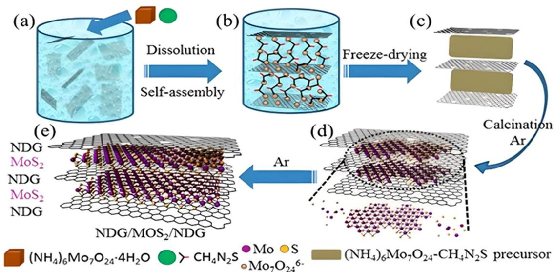
**Fig. 14** (a–e) Schematic representation of different steps involved in the synthesis of layer-by-layer NG/MoS<sub>2</sub>/NG stacking heterostructure. Reprinted with permission from ref. 93. Copyright 2017, Elsevier.
