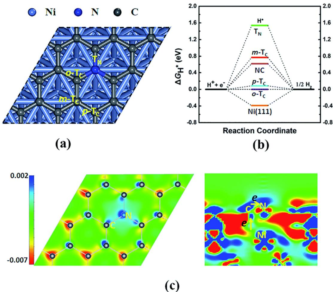
**Fig. 28** Typical electron transfer process Ni  $\rightarrow$  C  $\rightarrow$  N. (a) Theoretical model used in DFT calculations and obtained adsorption site of H\* on model surface. (b) Computed free energies for adsorption sites. (c) Charge density difference of the Ni(111)@NC model, where red and blue areas signify low and high electron density, respectively. Reprinted with permission from ref. 239. Copyright 2020, The Royal Society of Chemistry.
