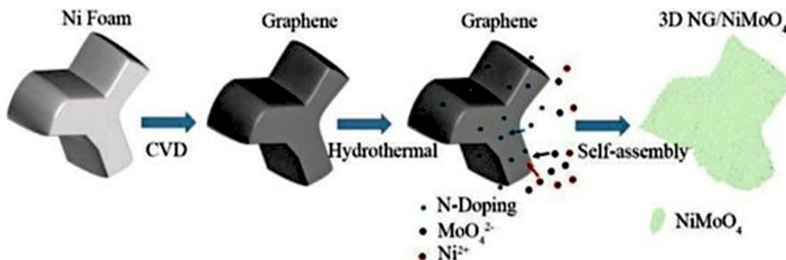
Fig. 10 Illustration of the fabrication process of NG/NiMoO<sub>4</sub>. Reprinted with permission from ref. 89. Copyright 2020, Elsevier.
