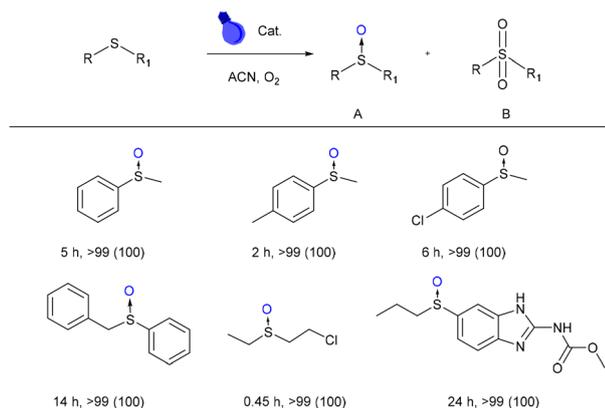
**Fig. 4** Photocatalytic performance in the sulfoxidation reaction (in parentheses, selectivity to sulfoxide). Conditions: catalyst (4.4 mg), sulfide (0.2 mmol), acetonitrile (0.5 mL), irradiated by blue LED light (2 × 30 W) at RT under an O<sub>2</sub> balloon atmosphere. Conversion and selectivity determined by GC-MS and <sup>1</sup>H-NMR.
