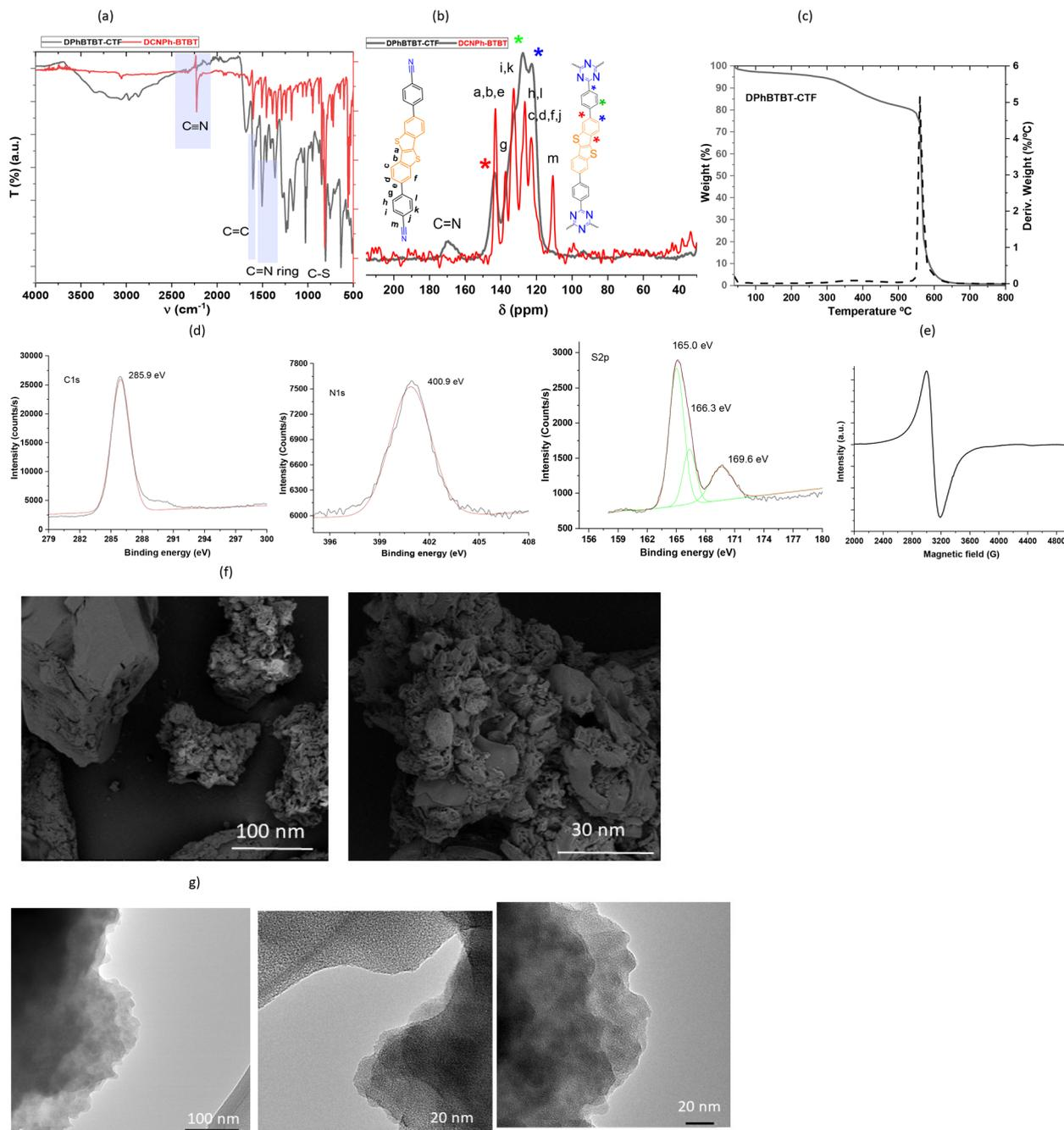
**Fig. 2** Characterization data: (a) FTIR spectra and (b) solid-state  $^{13}\text{C}$  NMR spectra of the monomer (red line) and **DPhBTBT-CTF** (black line), (c) TGA, (d) XPS traces, (e) EPR, (f) SEM and (g) TEM images of **DPhBTBT-CTF**.
