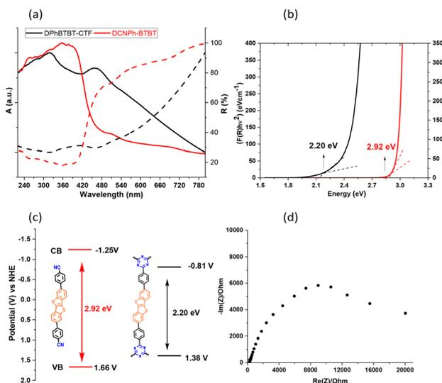
**Fig. 3** Top: (a) UV–Vis and diffuse reflectance spectra and (b) Tauc plots obtained with the Kubelka–Munk function and the linear fit for optical band gaps. Down: (c) HOMO and LUMO energy levels and (d) Nyquist plot (applied voltage  $E = 1.8 \text{ V}$ ).
