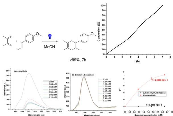
**Fig. 7** Top: D–A reaction between *trans*-anethole (0.13 mmol – 1 eq.) and 2,3-dimethyl-1,3-butadiene (0.4 mmol – 3 eq.) in 0.5 mL of ACN with 4.4 mg catalyst loading and kinetic profile. Down: Fluorescence quenching experiments.
