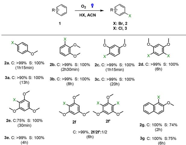
**Fig. 6** Photocatalyzed halogenation of aromatic compounds: substrate (0.15 mmol), HBr 47% (1.05 mmol) or HCl 37% (1.05 mmol), catalyst (4.4 mg), acetonitrile (0.5 mL), a LED blue lamp, r.t.; conversion was followed by GC and yields are determined by  $^1\text{H-NMR}$  (selected GC chromatograms and NMR spectra are shown in Fig. S15–S21 and S23–S27 $\dagger$ ).
