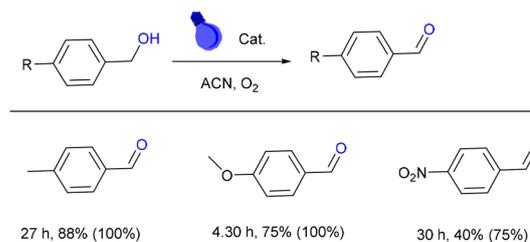
**Fig. 5** Photooxidation of benzylic alcohols (in parentheses, selectivity to aldehydes). Conditions: substrate (0.2 mmol), catalyst (4.4 mg), acetonitrile (0.5 mL), O<sub>2</sub> and blue LED light (2 × 30 W) (conversion and selectivity determined by GC-MS).
