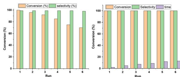
**Fig. 9** Left: Oxidation of mustard gas simulant in the presence of **DPhBTBT-CTF** under a blue LED with six consecutive injections of substrate. Right: Recycling of **DPhBTBT-CTF** toward mustard gas simulant.
