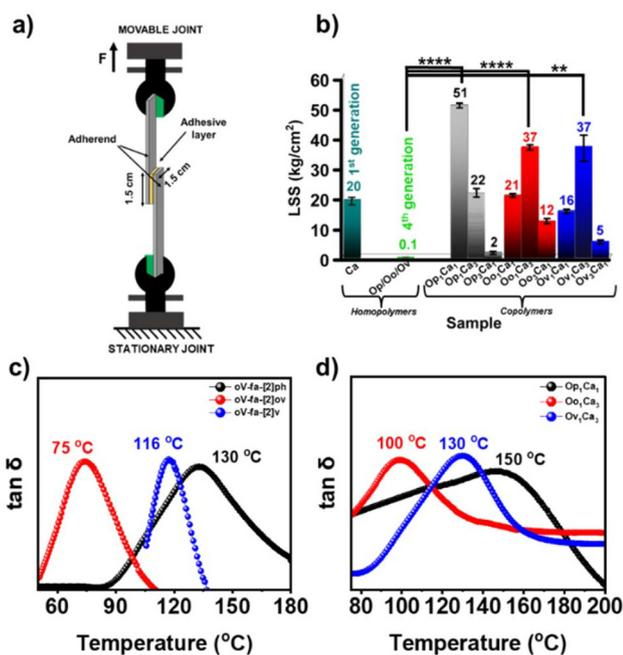
**Fig. 9** Mechanical properties. (a) Adhesive strength measurements. A schematic illustration of the LSS measurements using a polymer as the adhesive. (b) The adhesive strength of the homo- and copolymers determined at 35 °C. Bars display mean  $\pm$  S.E. \*\*\*\* $p$  < 0.0001 and \*\* $p$  < 0.0024. The dynamic mechanical thermal analysis study of samples. Damping factor ( $\tan \delta$ ) plots of (c) homopolymers and (d) copolymers.
