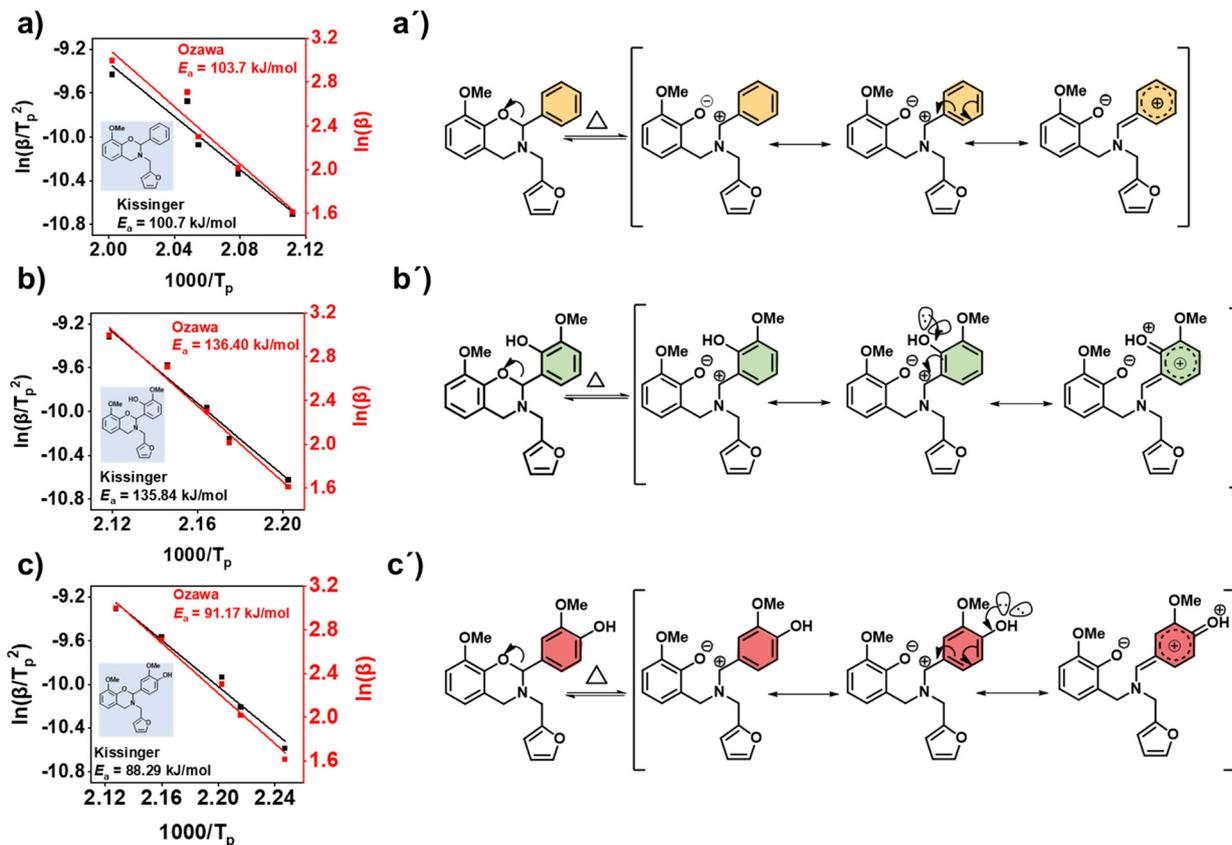
Fig. 7 (a–c) The plots of activation energy  $E_a$  calculated by the Kissinger–Akahira–Sunose (KAS) (black) and modified Ozawa (red) methods for the polymerization reaction. (a'–c') The stability of the ring-opened iminium ion intermediate due to charge delocalization in the functionalised un/substituted benzene structure in the respective monomer. For the sake of comparable analysis  $H_{\text{phenolic}}$  at  $C_2$  of benzene ring is not shifted to the hetero-atoms in the oxazine-ring.
