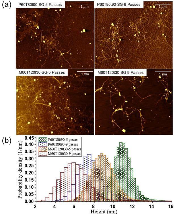
Fig. 11 AFM images of LCNFs from AHF WISs (a) using p-TsOH and MA and varied passes through microfluidization along with their AFM topography-measured (b) LCNF height probability distributions. <sup>50</sup> Copyright 2021 Elsevier.
