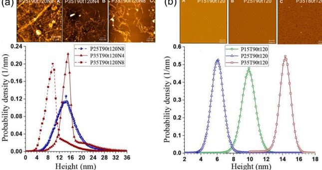
Fig. 10 Performance and application of p-TsOH using biomass processing. (a) atomic force microscopic (AFM) images of lignocellulosic nanofibrils (LCNFs) and AFM measured their height distributions, (b) AFM images of lignin nanoparticle (LNPs) and dynamic light scattering measured particle size distributions. 119 Adapted with permission from 119. Copyright 2018 American Chemical Society.
