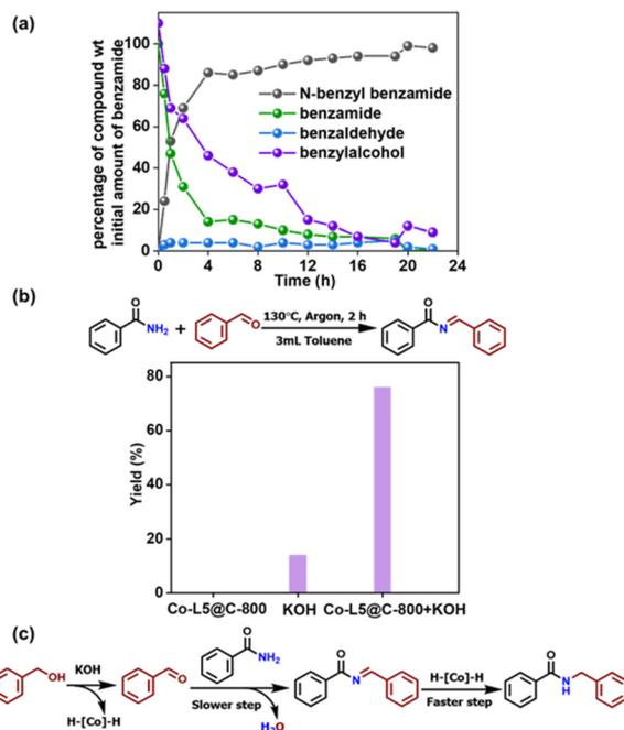
**Fig. 2** Kinetic experiment and control reactions. (a) Kinetic profile of the model reaction. Reaction conditions: 0.5 mmol of benzamide, 0.55 mmol of benzyl alcohol, 60 mg of catalyst, 1 atm argon, 3 mL of toluene, 130 °C, and GC yield. (b) Coupling reaction of benzamide and benzaldehyde to form secondary amide. Reaction conditions: same as (a) with 0.5 mmol of benzamide, 0.55 mmol of benzaldehyde, and 2 h. (c) Proposed reaction sequence.
