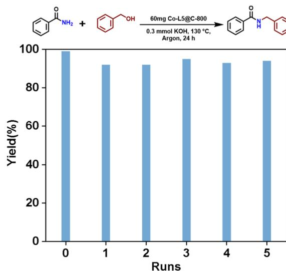
**Fig. 5** Reusability of Co-L5@C-800 in *N*-alkylation of benzamide with benzyl alcohol. Reaction conditions: 0.5 mmol benzamide, 0.55 mmol benzyl alcohol, 60 mg Co-L5@C-800 (1.9 mol% Co), 0.3 mmol KOH, 3 mL toluene, 130 °C, 24 h, in 1 atm argon.
