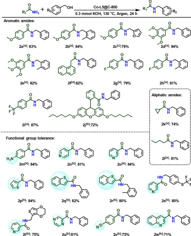
**Scheme 2** Co-L5@C-800 catalyzed *N*-alkylation of different amides with benzylic alcohol. Conditions: <sup>a</sup> 0.5 mmol of amide, 0.55 mmol of benzyl alcohol, 60 mg of Co-L5@C-800 (1.9 mol% Co), 0.3 mmol of KOH, 3 mL of toluene, 130 °C, 24 h, and in 1 atm argon. Isolated yields. <sup>b</sup> Same as [a] at 140 °C. <sup>c</sup> Same as [a], GC yield.
