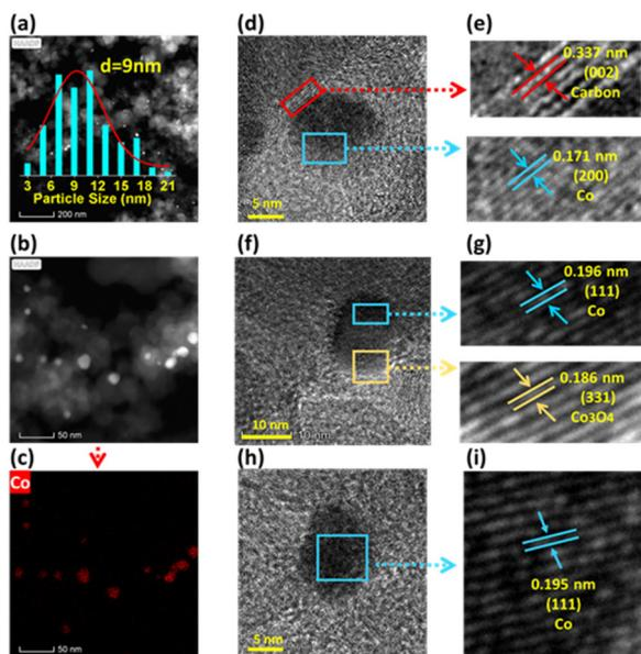
**Fig. 4** TEM analysis of Co-L5@C-800. (a and b) TEM-HAADF images, (c) EDX elemental mapping image of Co, and (d–i) identified crystal planes of the Co nanoparticles.
