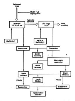
Fig. 3 The organocell process (reproduced from ref. 69 with permission from *Tappi J.*, copyright 1989).
