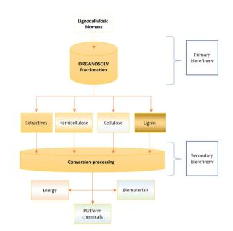
Fig. 1 Organosolv fractionation in biorefinery.
