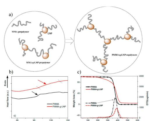
Fig. 6 (a) Schematic image of the polymerization process. (b) DSC scan of PMMA and PMMA-g-LNP. (c) TGA and DTG curves of PMMA and PMMAg-LNP.<sup>21</sup> (a-c) Were reproduced with permission from Yang, 2018, Copyright (2018) Elsevier.
