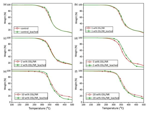
Fig. 4 The Thermogravimetric analysis (TGA) curves of (a) control, (b) 1 wt% OSL/NR, (c) 2 wt% OSL/NR, (d) 5 wt% OSL/NR, (e) 10 wt% OSL/NR and (f) 20 wt% OSL/NR samples, with and without dusting and leaching processes. <sup>76</sup> (a-f) were reproduced with permission from Hosseinmardi, 2021, Copyright (2021) Elsevier.
