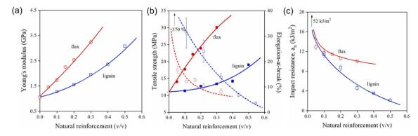
Fig. 16 Different mechanical properties of PP composites blended with various concentrations of flax (O) and lignin ( $\square$ ), reproduced with permission from Pregi, 2022, Copyright (2022) Elsevier. 154
