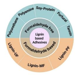
Fig. 2 Lignin-based adhesives are divided into two categories, i.e., lignin-based formaldehyde resins and lignin-based formaldehyde-free
