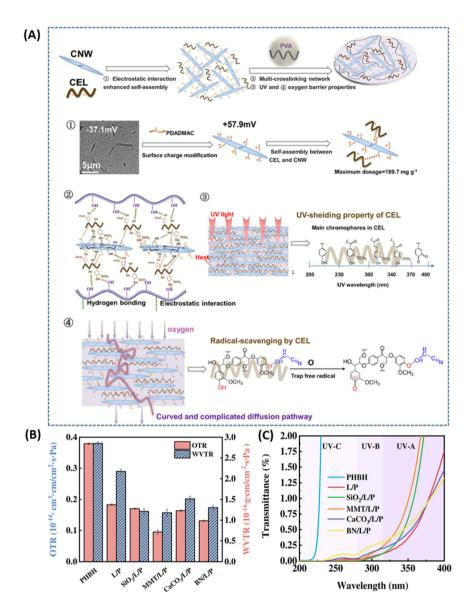
Fig. 10 (A) Schematic diagram showing the procedure of composite film production and its structural details leading to UV and oxygen shielding, reproduced with permission from Tian, 2023, Copyright (2023) Elsevier. (B) OTR, WVTR performance and (C) UV-visible spectra of PHBH, lignin/PHBH (L/P), and INPs incorporated composites, reproduced with permission from Zeng, 2022, Copyright (2022) Wiley.
