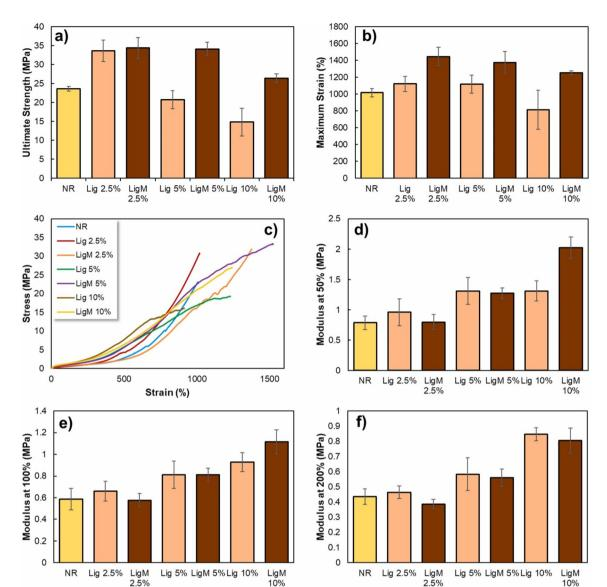
Fig. 18 Tensile analysis of baseline natural rubber and its composites with lignin and modified lignin at various concentrations, (a) Ultimate strength, (b) Elongation at break, (c) Stress-strain plots, (d) Elastic modulus at 50%, (e) Elastic modulus at 100% and (f) Elastic modulus at 200%, reproduced with permission from Shorey, 2021, Copyright (2021) Elsevier.<sup>170</sup>
