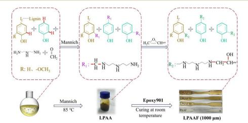
Fig. 17 Schematic illustration of black liquor lignin-based phenolic amine synthesis and epoxy composite preparation, reproduced with permission from Li, 2023, Copyright (2023) Elsevier.<sup>163</sup>
