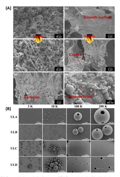
Fig. 11 (A) Morphology of PGM-3 aerogel before and after flame tests. PGM-3 aerogel showing (a) original microstructure and (b) smooth surface before, and (c and d) rough surface after flame tests. (f) The nanoparticles surfaced on the aerogel after flame tests, reproduced with permission from Li, 2022, Copyright (2022) Elsevier. (B) SEM images of LNPs obtained from various lignin fractions, reproduced with permission from Zhang, 2023, Copyright (2023) Elsevier.
