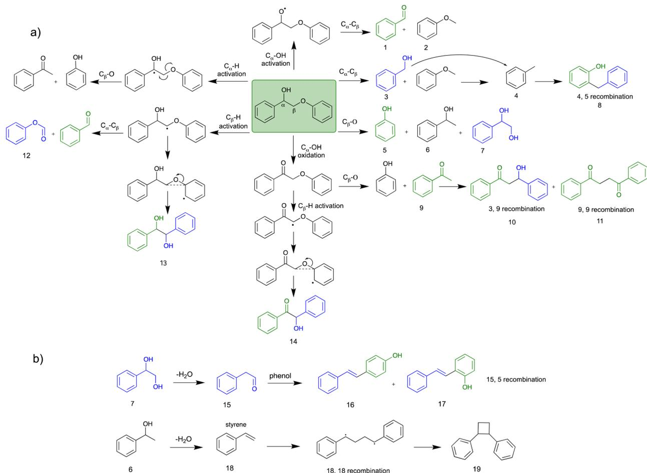
**Scheme 2** The proposed mechanism for the conversion of PPE using electrochemical oxidation under a continuous flow microreactor in EtOH-water co-solvent system. (a) PPE conversion mechanism and (b) conversion of products 6 and 7.
