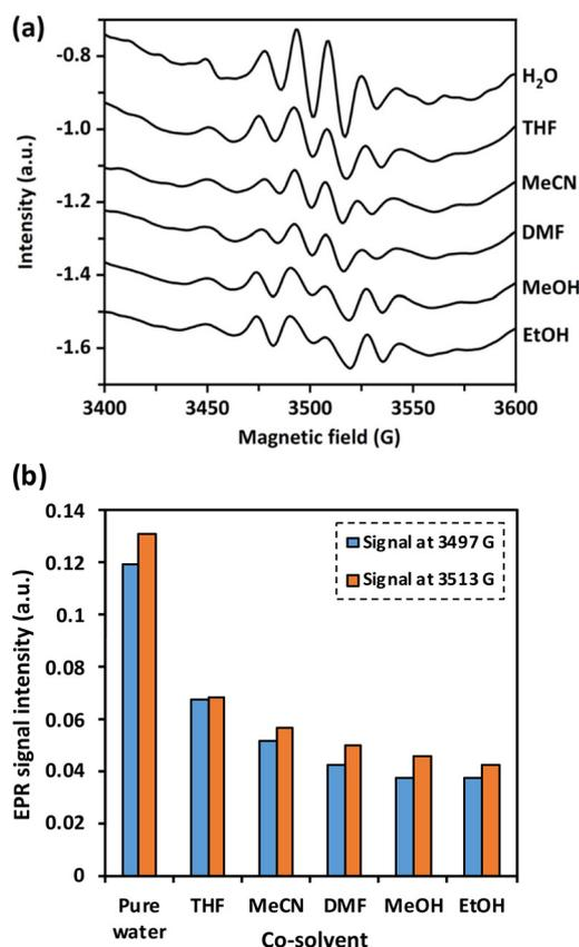
Fig. 2 Effect of OH radical scavenger in different co-solvent systems (reaction conditions: co-solvent, 30% vol. in water; H<sub>2</sub>O<sub>2</sub>, 500 ppm; DMPO, 500 ppm; and UV light irradiation for 20 min); (a) EPR spectra, (b) intensities of EPR signal corresponding to OH radicals.
