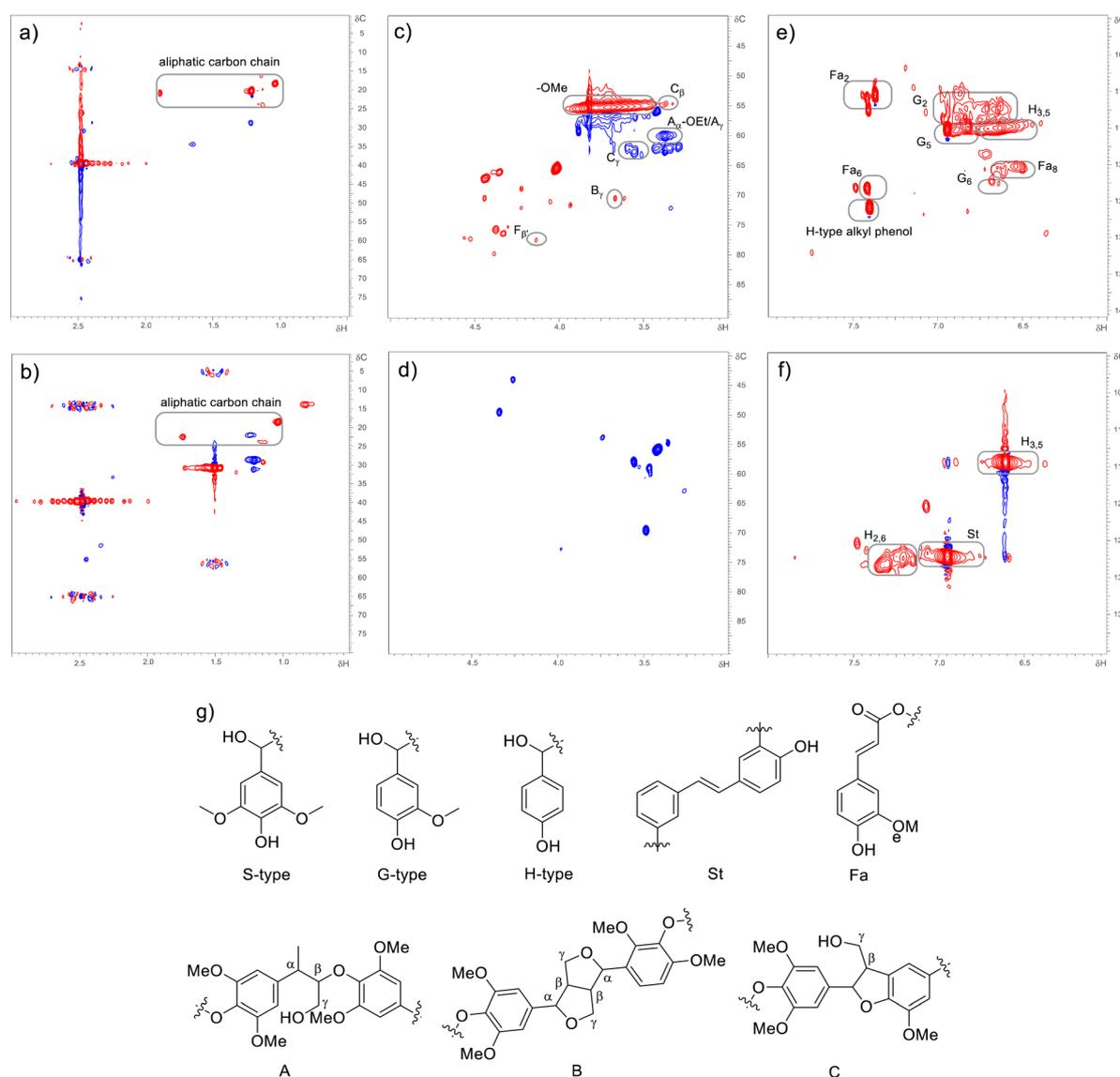
**Fig. 6** 2D-HSQC NMR (800 MHz) analysis of dealkaline lignin (a, c, and e) and depolymerization products of dealkaline lignin (b, d, and f). Reaction conditions: MeCN, 30% v in water; dealkaline lignin, 130 ppm; and applied current, 1 mA. Sub-aromatic units of lignin structure (g).
