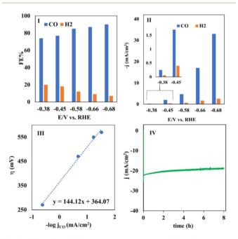
Fig. 6 (I) The FE and (II) partial current density of CO and H<sub>2</sub> measured in the electrolysis of CO<sub>2</sub> at different potentials using CoPc@GIOMC (0.9%) in the same solution as mentioned in Fig. 4I. (III) A plot of  $\eta$  vs.  $-\log j_{CO}$  for CO production in the electrolysis of CO<sub>2</sub> using CoPc@GIOMC (0.9%) at various overpotentials in 0.5 M KHCO<sub>3</sub>, and (IV) the recorded current density during 8 h electrolysis of CO<sub>2</sub> at -0.66 V vs. RHE.
