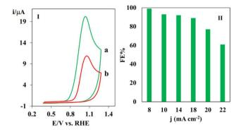
Fig. 8 (I) The cyclic voltammograms of the anodic part of the paired electrolysis (a) at the start and (b) after 135 minutes electrolysis in a twoelectrode set-up at 14 mA cm<sup>-2</sup> containing catechol and TSA in the anodic part, and (II) the plot of FE% vs. current density for the anodic part of the electrolysis mentioned in part I.
