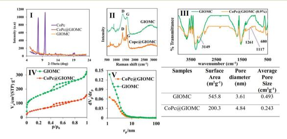
Fig. 3 (I) The XRD pattern of pure CoPc, CoPc@GIOMC (0.9%) hybrid, and pure GIOMC. (II) The Raman spectra, (III) FTIR spectra, (IV) N2 adsorption-desorption isotherm, and (V) pore size distribution of GIOMC and the CoPc@GIOMC (0.9%) hybrid. Table: surface area, pore diameter, and average pore size of GIOMC and the CoPc@GIOMC (0.9%) hybrid.
