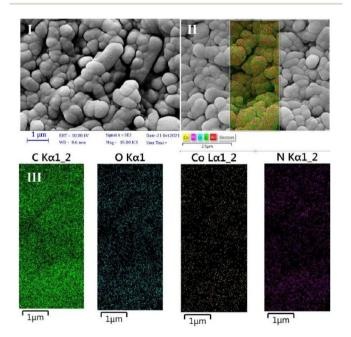
Fig. 1 The SEM images of (I) GIOMC, (II) CoPc@GIOMC (0.9%) hybrid, and (III) elemental mapping analysis of C, O, N, and Co.
