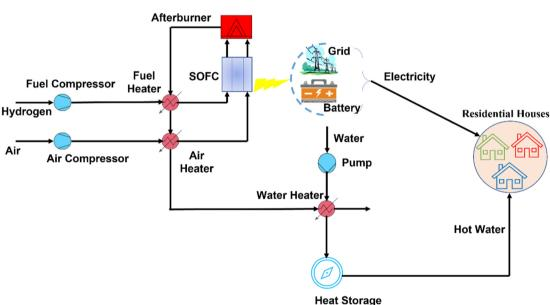
Fig. 2 Schematic of SOFC integrated CHP system fuelled by (a) natural gas and (b) hydrogen.
