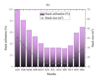
Fig. 11 SOFC stack utilisation based on monthly requirement for SOFC—heat pump fuelled by (a) NG (b)  $\rm H_2$ .
