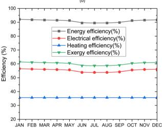
**Fig. 5** Efficiency of the SOFC-based system on monthly basis fuelled by (a) NG (b) hydrogen.
