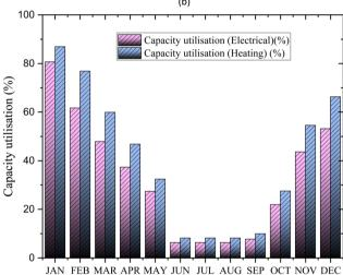
**Fig. 6** Capacity utilisation of the proposed SOFC-based system on monthly basis fuelled by (a) NG, (b) hydrogen.
