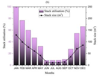
Fig. 7 SOFC stack utilisation based on monthly requirement for (a) NG based system (b) H<sub>2</sub> based system.
