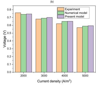
Fig. 4 (a) Comparison of model and experimental data for a single cell of SOFC fuel cell using 1000 °C with 89%  $\rm H_2$  and 11%  $\rm H_2O$  as fuel. (b) Comparison of present model, numerical model<sup>45</sup> and experimental data, <sup>46</sup> with CH<sub>4</sub> as fuel.
