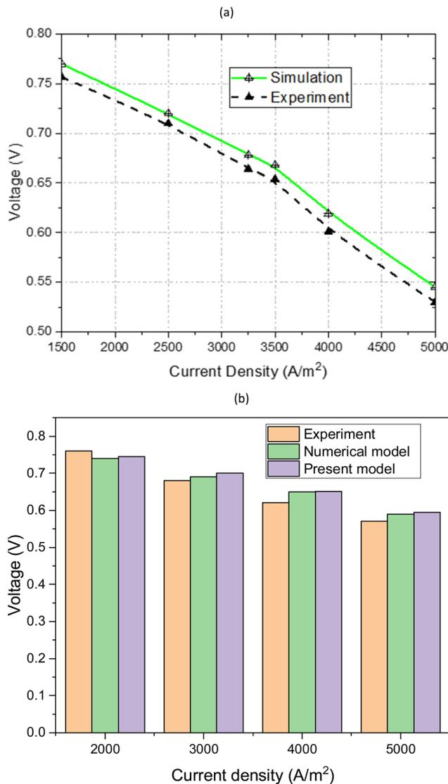
Fig. 4 (a) Comparison of model and experimental data for a single cell of SOFC fuel cell using 1000 °C with 89% H<sub>2</sub> and 11% H<sub>2</sub>O as fuel. (b) Comparison of present model, numerical model<sup>45</sup> and experimental data,<sup>46</sup> with CH<sub>4</sub> as fuel.
