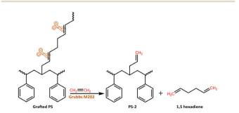
Scheme 2 Schematic representation of the ethenolysis-metathesis using the rubber phase as a starting material.
