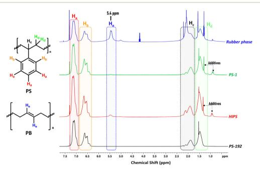
Fig. 4 <sup>1</sup>H-NMR comparison of commercial PS-192, HIPS, PS-1 (isolated PS), and the rubber phase. The spectra illustrate the most distinctive proton signals of both polymers contained in HIPS (400 MHz, solvent CDCl<sub>3</sub>).
