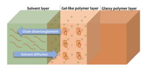
Fig. 2 Representation of the polymer dissolution process.<sup>59</sup>
