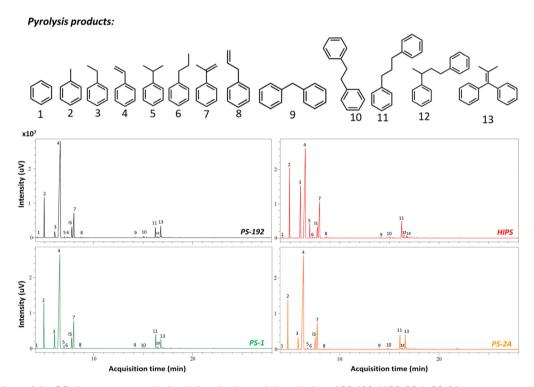
Fig. 8 Comparison of the GC chromatograms obtained after the thermal degradation of PS-192, HIPS, PS-1, PS-2A.
