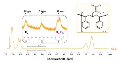
Fig. 6 <sup>1</sup>H-NMR spectrum of PS-2 isolated from the ethenolysis reaction mixture (600 MHz, solvent CDCl<sub>3</sub>).
