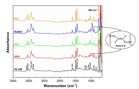
Fig. 7 ATR-FTIR spectra of PS-192, HIPS, PS-1, PS-2 and the rubber phase. Major differences are observed in the intensity of the 964 cm<sup>-1</sup> band, attributed to the C=C vibration of *trans*-1,4 double bonds.
