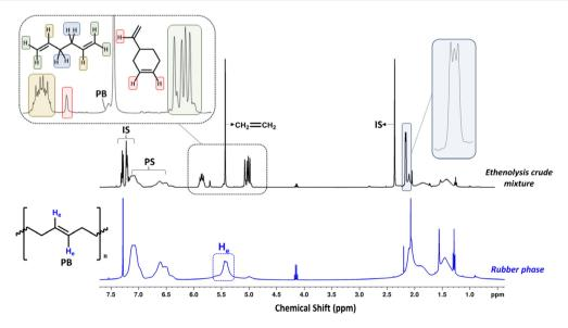
Fig. 5 <sup>1</sup>H-NMR comparison of the rubber phase and the crude ethenolysis reaction mixture. Signals at 7.3, 7.2, 2.4 ppm in the ethenolysis crude reaction mixture spectrum correspond to toluene (internal standard), while the signal at 5.4 ppm corresponds to leftover ethylene gas (400 MHz, CDCl<sub>3</sub>).
