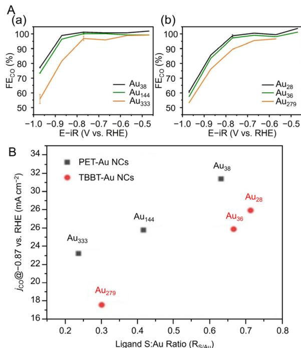
**Fig. 19** (A)  $FE_{CO}$  of (a) PET-protected  $Au_{38}$ ,  $Au_{144}$  and  $Au_{333}$  and (b) TBBT-protected  $Au_{28}$ ,  $Au_{36}$  and  $Au_{279}$  NCs. (B) Electrochemical performance:  $j_{CO}$  (at  $-0.87$  V vs. RHE) vs. S : Au ratio of  $Au_{38}$ ,  $Au_{144}$ ,  $Au_{333}$  and  $Au_{28}$ ,  $Au_{36}$ ,  $Au_{279}$  series of NCs (A) and (B) are reproduced with permission from ref. 296. Copyright 2022 Wiley-VCH GmbH.
