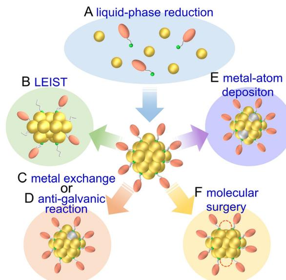
**Fig. 33** Schematic of the synthesis methods of metal NCs using (A) liquid-phase reduction, (B) ligand-exchange-induced size/structure transformation (LEIST), (C) metal exchange, (D) anti-galvanic reaction, (E) metal-atom deposition, (F) molecular surgery.
