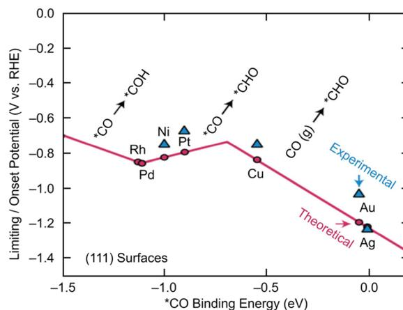
**Fig. 16** A volcano plot of CO<sub>2</sub> reduction reactions for (111) bulk metals. This figure is reproduced with permission from ref. 279. Copyright 2017 AAAS.
