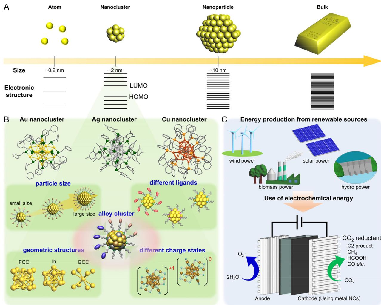
**Fig. 1** Schematic of this review. A next-generation energy system based on electrocatalytic CO<sub>2</sub> reduction reaction using metal-cluster catalysts. (A) Size dependences of metals for electronic structure; (B) kinds of metal clusters and each parameter for electrocatalytic CO<sub>2</sub> reduction reaction; and (C) a flow reaction system for electrocatalytic CO<sub>2</sub> reduction using electricity from renewable energy source.
