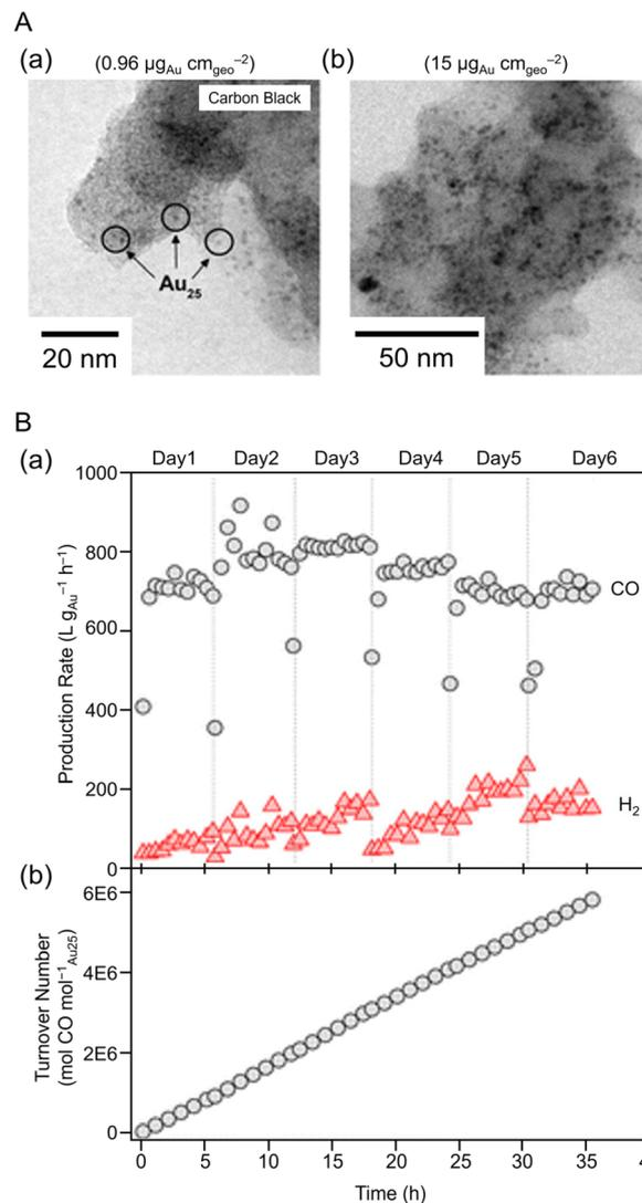
**Fig. 18** (A) TEM images of carbon-supported Au<sub>25</sub> at low and high loadings. Isolated 1.4 ± 0.4 nm Au NC were observed on the carbon black support at low loadings. (B) Day-to-day (a) product formation rates, (b) cumulative TON (mol of CO/mol of Au<sub>25</sub>). Panels (A) and (B) are reproduced with permission from ref. 293. Copyright 2015 American Chemical Society.
