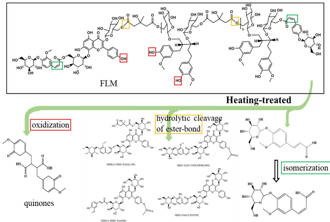
**Fig. 3** Schematic of the structural changes of FLMs after heat treatment (ChemDraw Ultra 14.0). The reactive site and type are marked in red (oxidation), yellow (depolymerization) and green (isomerization).
