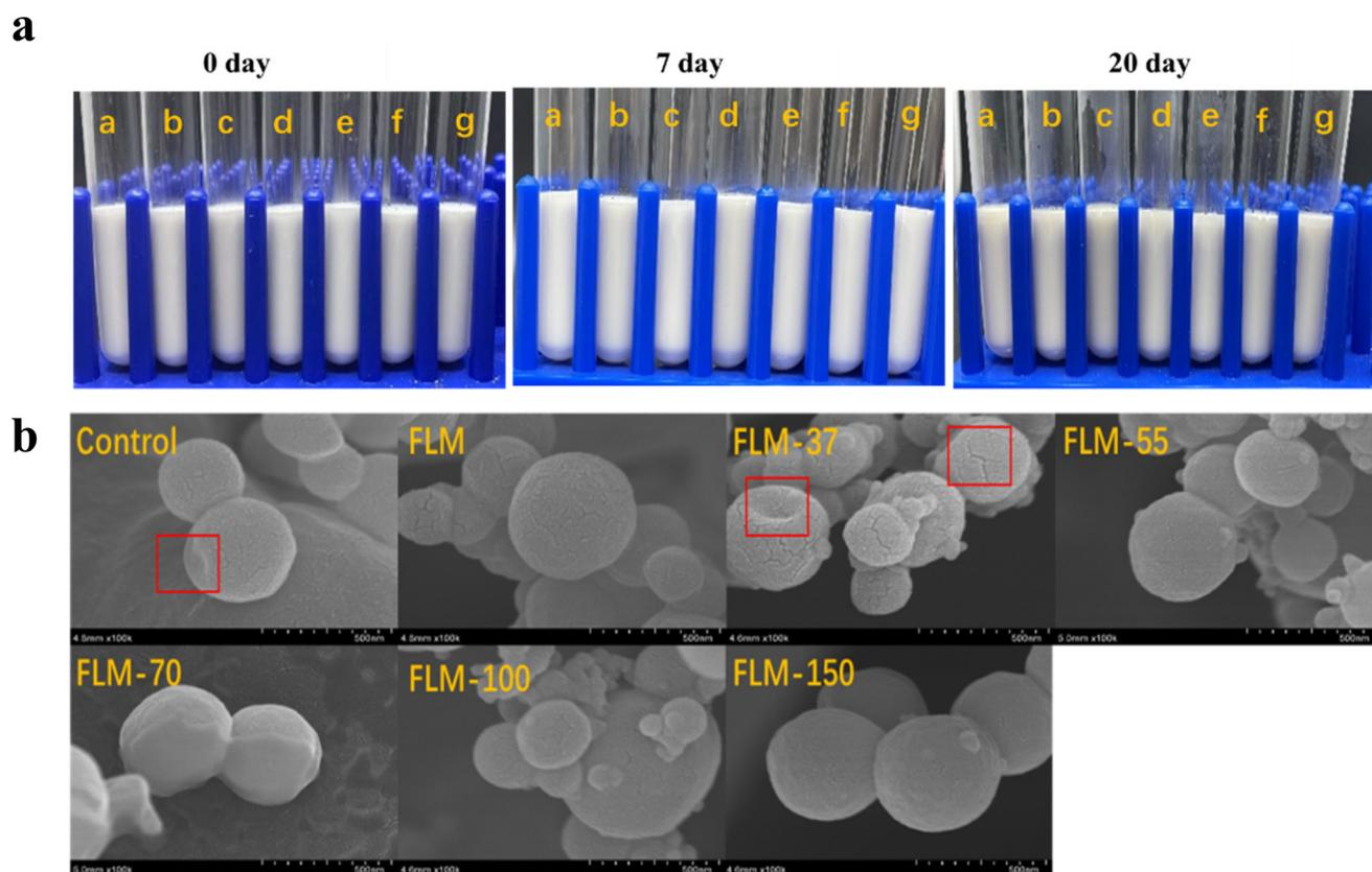
**Fig. 6** (a) Appearance of emulsions (0, 7 and 20 d), (letters a–g represent FLM, FLM-37, FLM-55, FLM-70, FLM-100, and FLM-150). (b) The morphology observations of emulsions using cryo-scanning electron microscopy (0 d).
