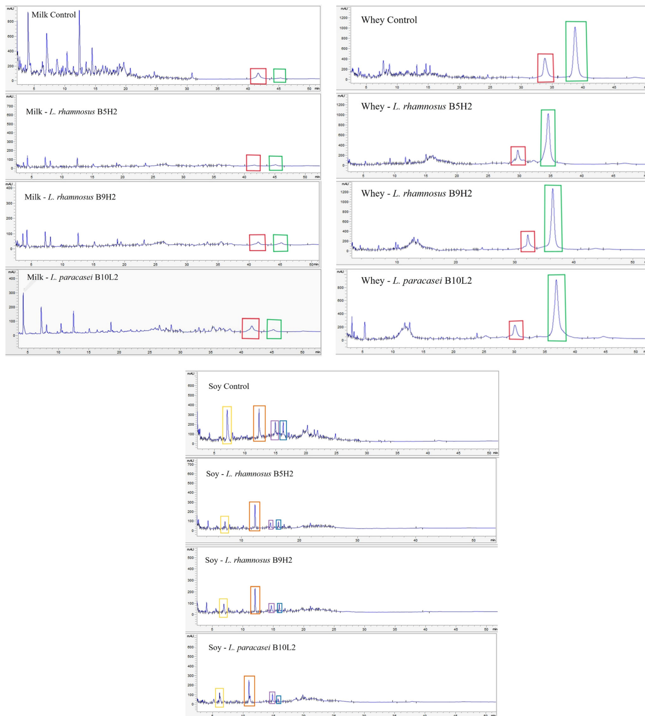
Fig. 5 (a) HPLC-DAD chromatograms of milk samples; control (non-fermented) and fermented by L. rhamnosus B5H2, L. rhamnosus B9H2 and L. paracasei B10L2. Alpha-lactoglobulin (red frame) and beta-lactoglobulin (green frame) are highlighted. (b) HPLC-DAD chromatograms of whey samples; control (non-fermented) and fermented by L. rhamnosus B5H2, L. rhamnosus B9H2 and L. paracasei B10L2. Alpha-lactoglobulin (red frame) and beta-lactoglobulin (green frame) are highlighted. (c) HPLC-DAD chromatograms of soy samples; control (non-fermented) and fermented by L. rhamnosus B5H2, L. rhamnosus B9H2 and L. paracasei B10L2. Major protein peaks are highlighted.
