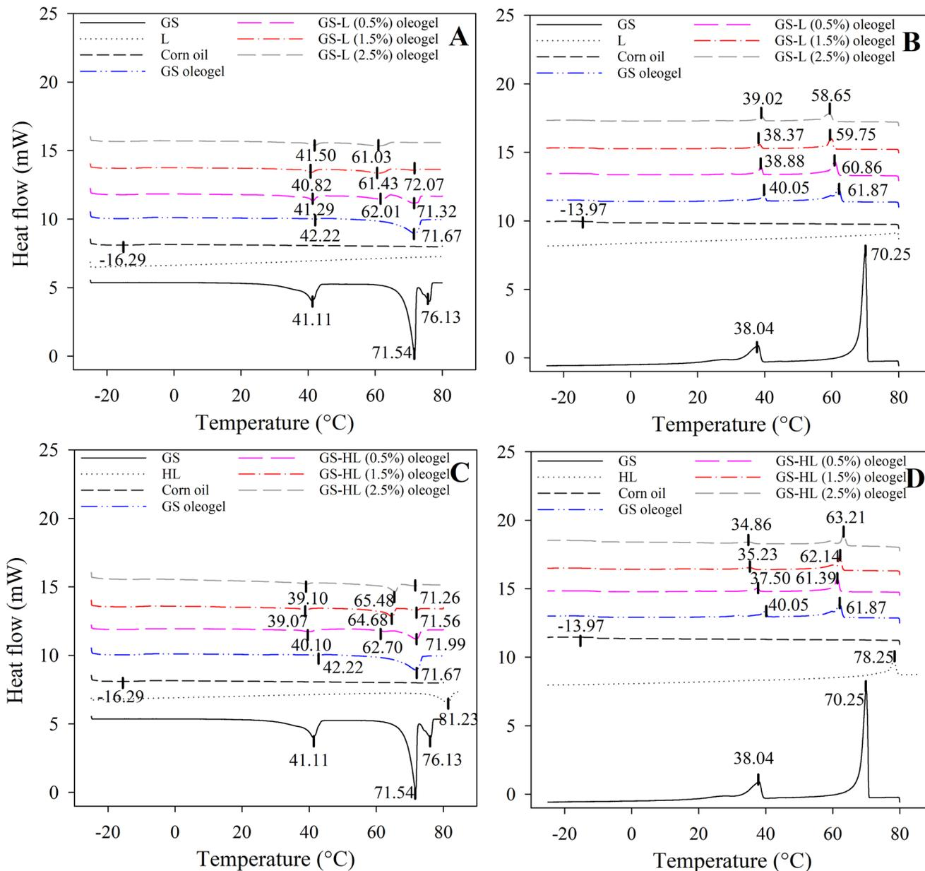
**Fig. 1** DSC profiles of the neat lecithin (L), neat hydrogenated lecithin (HL), neat glyceryl stearate (GS), liquid corn oil and corn oil-based oleogels containing GS, lecithin or hydrogenated lecithin at concentrations of 0.5, 1.5 and 2.5% (w/w) with second heating cycles for lecithin-containing oleogels (A) and hydrogenated lecithin-containing oleogels (C), and cooling cycles for lecithin-containing oleogels (B) and hydrogenated lecithin-containing oleogels (D).
