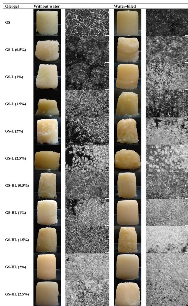
**Fig. 2** Photos and polarized light microscopic images of corn oil oleogels at 25 °C (left column) and their water-filled counterparts (right column) for glyceryl stearate (GS) oleogels, lecithin (L)-containing oleogels, and hydrogenated lecithin (HL)-containing oleogels. The scale bar corresponds to 100  $\mu\text{m}$ .
