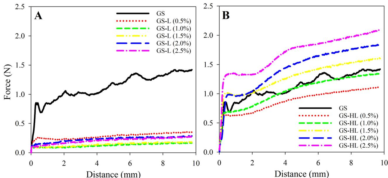
Fig. 4 Penetration force (N) of corn oil oleogels over a distance of 10 mm at  $25.0 \pm 0.1$  °C for mixed systems with glyceryl stearate (GS) 20% (w/w) and different concentrations (0 to 2.5% w/w) of lecithin (L) (A) or hydrogenated lecithin (HL) (B).
