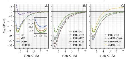
Fig. 2 The full binding curve for CO adsorption on the MgO (001) surface calculated using selected (A) wavefunction and (B and C) DFT methods. The energy data are denoted by the markers. The solid curves are obtained by fitting the data to the Morse potential. The inset in panel (A) shows a zoomed-in view for d(Mg-C) ranging from 2.25 to 2.75 Å.
