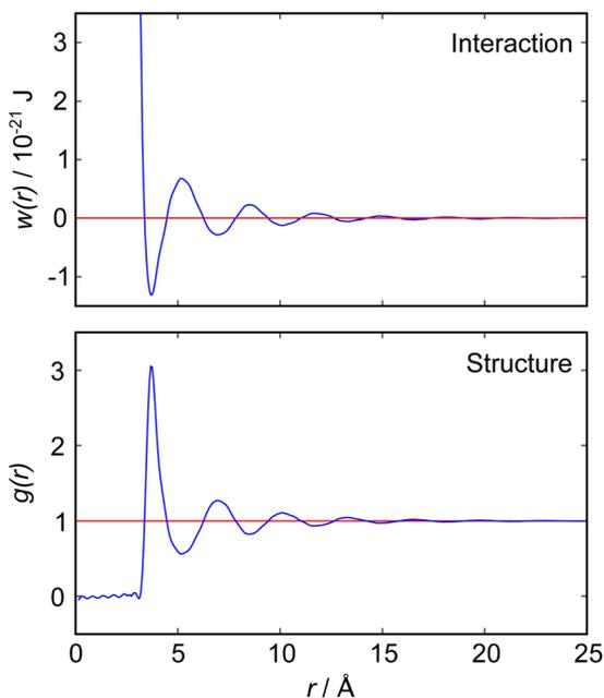
Fig. 1 (Bottom) Radial distribution function,  $g(r)$ , for liquid argon at 85 K, as measured by neutron scattering measurements by Yarnell *et al.*<sup>4</sup> (Top) Pair potential of mean force,  $w(r)$ , derived from the measured  $g(r)$  according to eqn (1). Both functions reveal a single damped oscillatory decay mode with a wavelength close to the argon atomic diameter.
