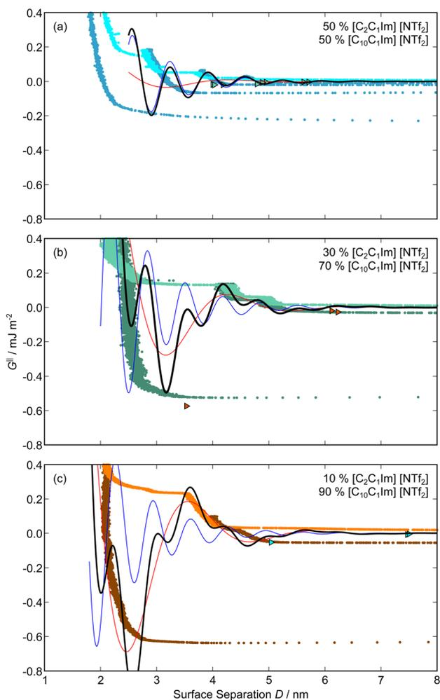
**Fig. 6** Interaction–distance profiles of ionic liquid mixtures, with fits as described in eqn (7) overlaid. The total fit is shown in black, with the contribution to the total fit from the charge ordering mode of  $[\text{C}_2\text{C}_1\text{Im}][\text{NTf}_2]$  shown in blue and the contribution from the bilayer mode of  $[\text{C}_{10}\text{C}_1\text{Im}][\text{NTf}_2]$  shown in red.
