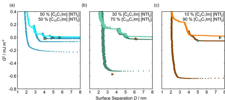
Fig. 5 Interaction–distance profiles of ionic liquid mixtures. Shown are measurements for (a): 50 mol%, (b): 30 mol%, and (c): 10 mol%  $[\text{C}_2\text{C}_1\text{Im}][\text{NTf}_2]$  in  $[\text{C}_{10}\text{C}_1\text{Im}][\text{NTf}_2]$ . Interactions measured on approach of the SFB surfaces are shown in the lighter colour while retractions are shown in the darker colour. Individual measurements of minima positions are shown as triangles.
