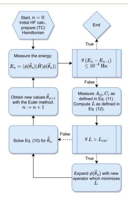
Fig. 4 The iteration procedure for TC-AVQITE.
